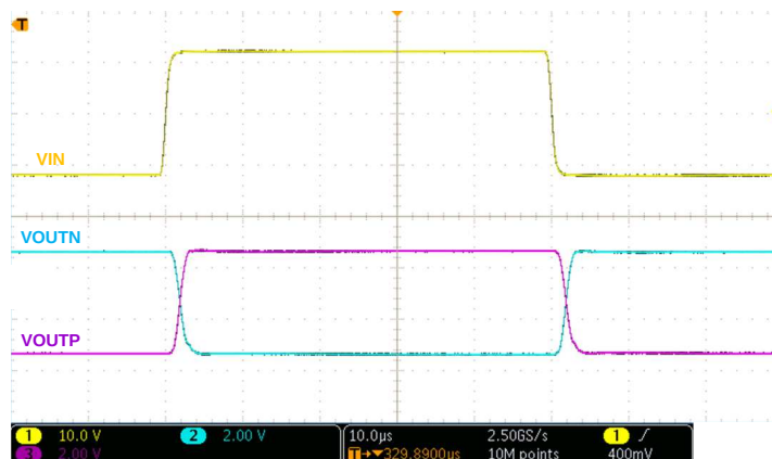
图 49. Step Response of the ISO224
