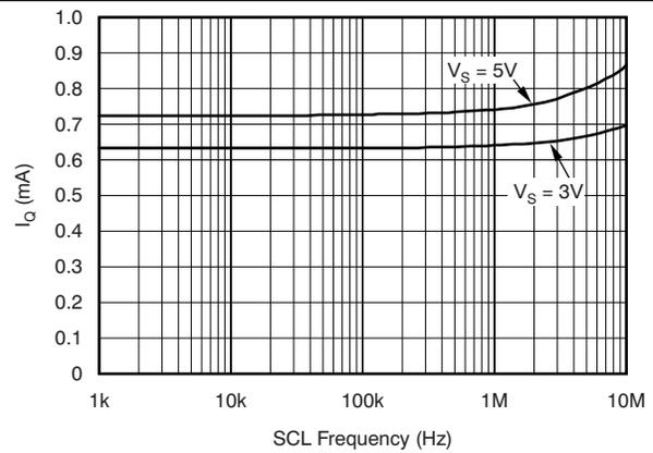
Figure 11. Active  $I_Q$  vs Two-Wire Clock Frequency
