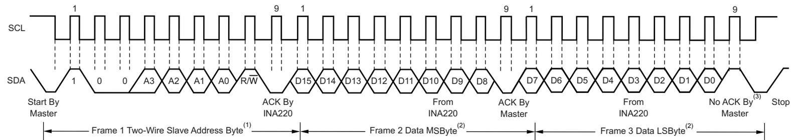
NOTES: (1) The value of the Slave Address Byte is determined by the settings of the A0 and A1 pins. Refer to Table 1.
