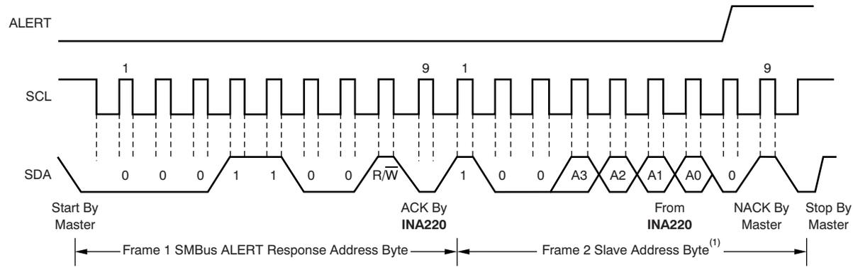
NOTE (1): The value of the Slave Address Byte is determined by the settings of the A0 and A1 pins. Refer to Table 1.
