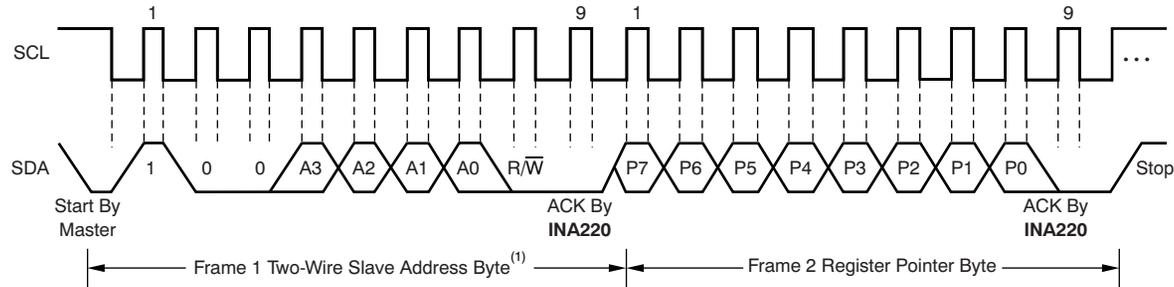
NOTE (1): The value of the Slave Address Byte is determined by the settings of the A0 and A1 pins. Refer to Table 1.
