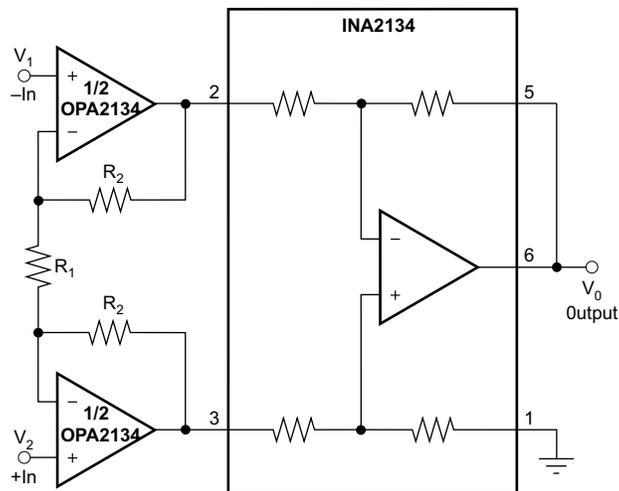
$$V_0 = (1 + 2R_2/R_1) (V_2 - V_1)$$
