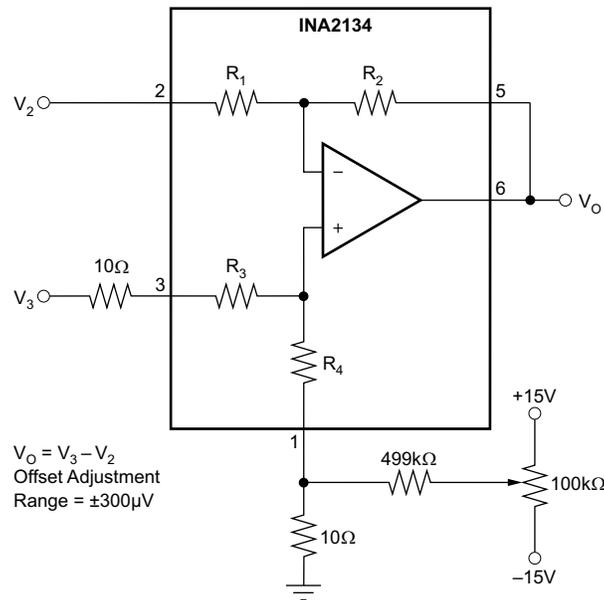
**Figure 3. Offset Adjustment**
