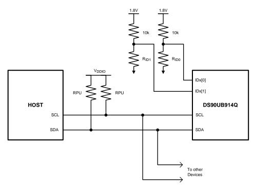
Figure 32. ID[x[ Address Decoder on the Deserializer
