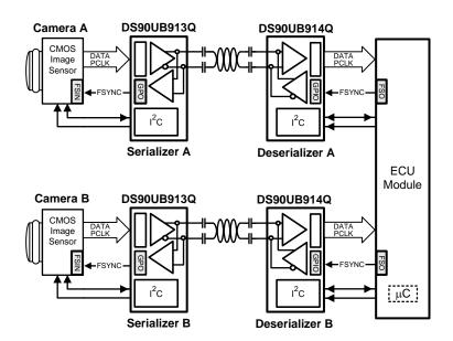
Figure 33. Synchronizing Multiple Cameras
