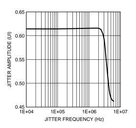
Figure 23. Typical Deserializer Input Jitter Tolerance Curve at 1.4-Gbps Line Rate
