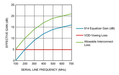
Figure 49. Adaptive Equalizer – Interconnect Loss Compensation
