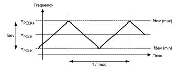
Figure 24. Spread Spectrum Clock Output Profile
