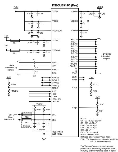
Figure 48. DS90UB914Q-Q1 Typical Connection Diagram — Pin Control
