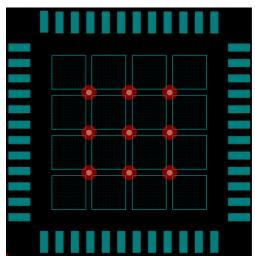
Figure 51. 48-Pin WQFN Stencil Example of Via and Opening Placement
