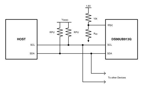
Figure 31. ID[x] Address Decoder on the Serializer
