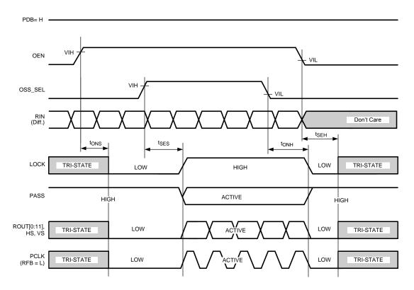
Figure 21. Output State (Set-Up and Hold) Times
