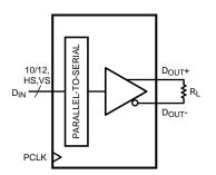
Figure 9. Serializer VOD Diagram
