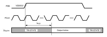
Figure 14. Serializer PLL Lock Time
