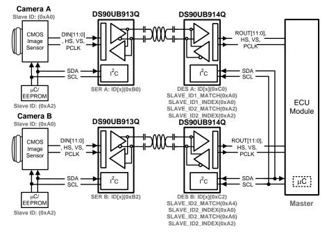
Figure 40. Multiple Device Addressing
