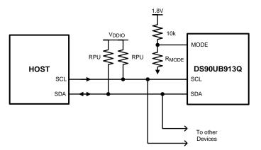
Figure 38. MODE Pin Configuration on DS90UB913Q-Q1
