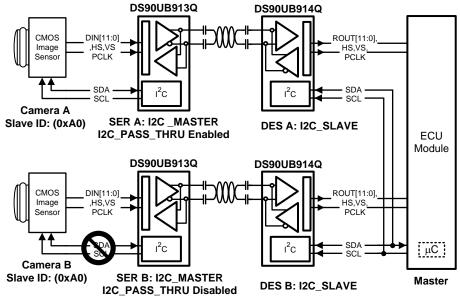
Figure 30. I<sup>2</sup>C Pass-Through
