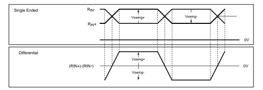
Figure 11. Differential Vswing Diagram
