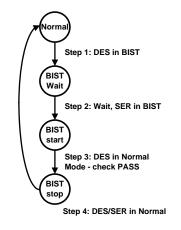
Figure 43. AT-Speed BIST System Flow Diagram
