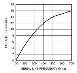
Figure 35. Maximum Equalizer Gain vs. Line Frequency
