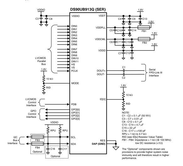
Figure 47. DS90UB913Q-Q1 Typical Connection Diagram — Pin Control
