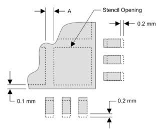
Figure 50. No Pullback WQFN, Single Row Reference Diagram
