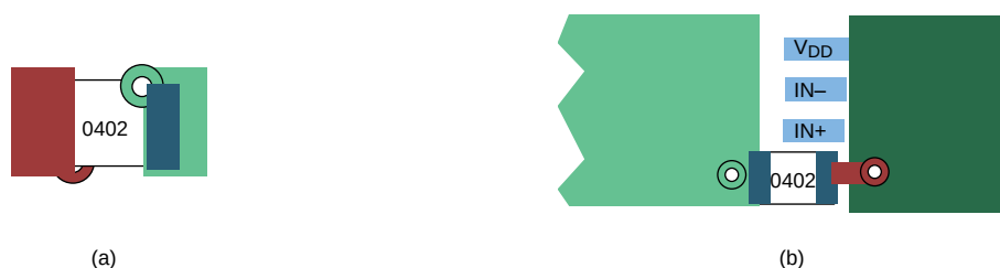
Figure 27. Typical Decoupling Capacitor Layouts
