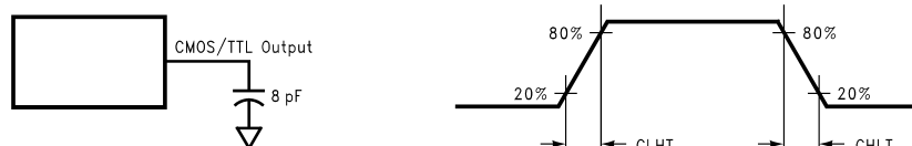
Figure 4. Receiver CMOS/TTL Output Load and Transition Times
