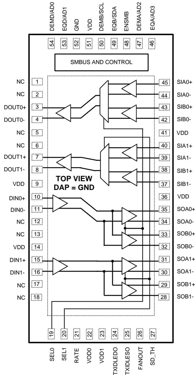
The center DAP on the package bottom is the device GND connection. This pad must be connected to GND through multiple (minimum of 4) vias to ensure optimal electrical and thermal performance.
