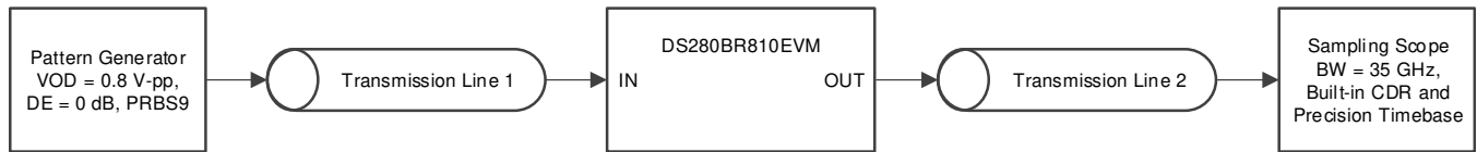
图 20. 10 in Rx and 5 in Tx Channel Test Setup
