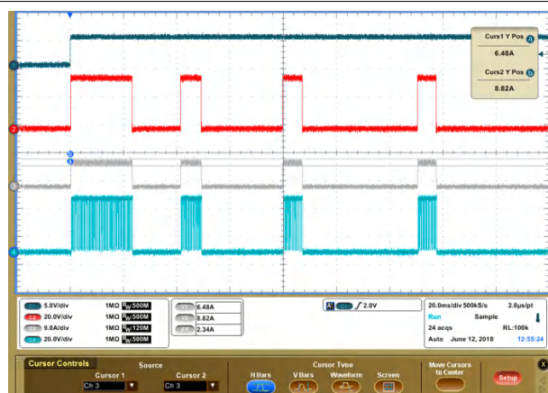
图 8-9. ITRIP Across TOFF and Load Current
