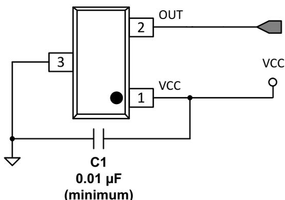
Figure 12. Typical Application Schematic – No Filter
