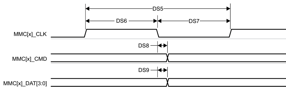
图 6-98. MMC1/2 – Default Speed – Transmit Mode
