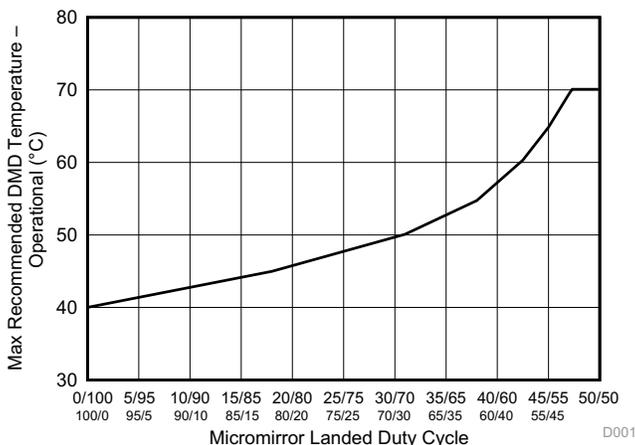
**Figure 1. Max Recommended DMD Temperature – Derating Curve**
