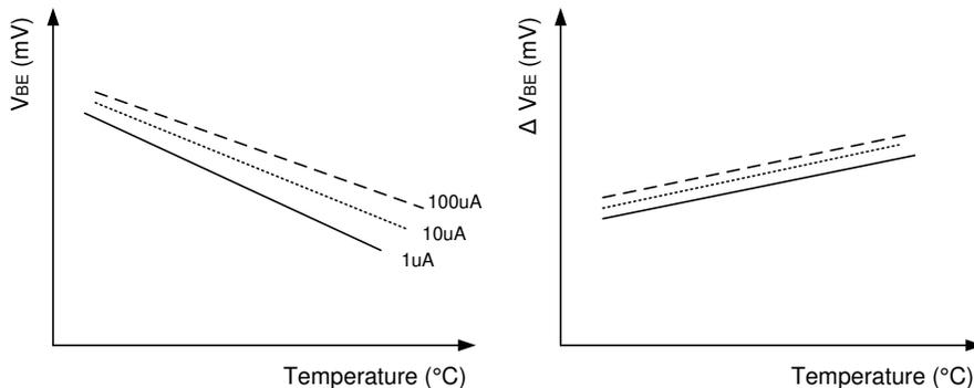
图 7-3. Example of Delta VBE vs. Temperature
