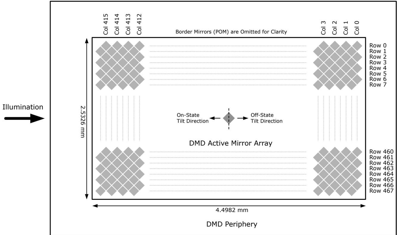
图 6-5. Micromirror Array Physical Characteristics
