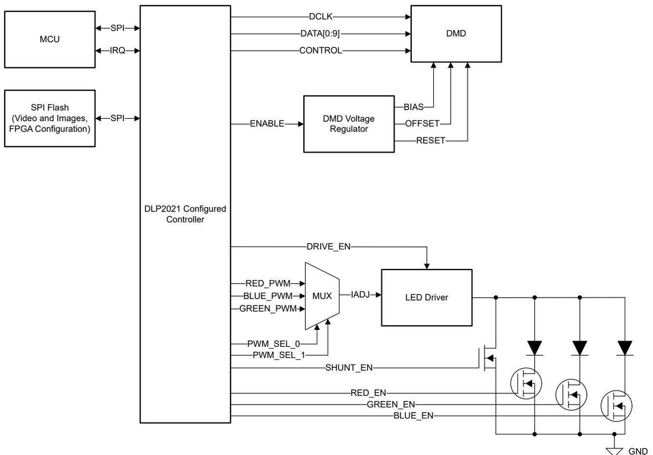
图 8-1. Dynamic Ground Projection System Block Diagram
