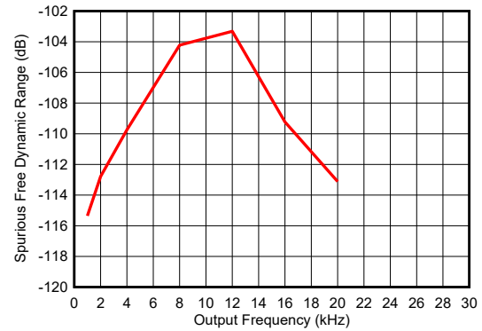
图 6-46. Spurious Free Dynamic Range vs Output Frequency, f_{DAC} = 768\text{ kHz}
