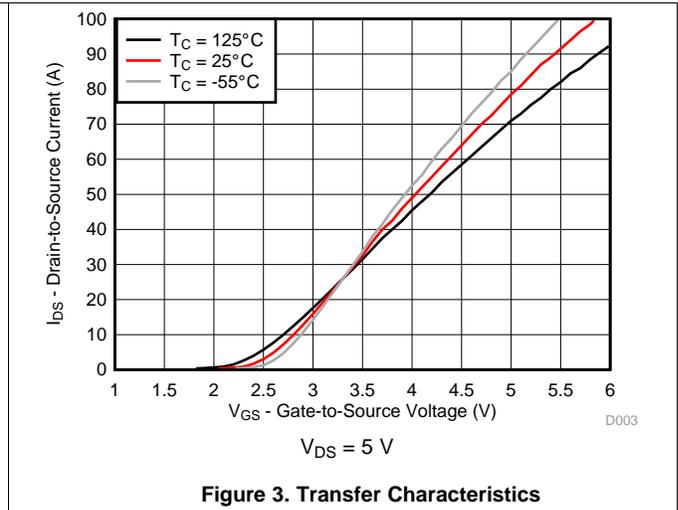
Figure 3. Transfer Characteristics
