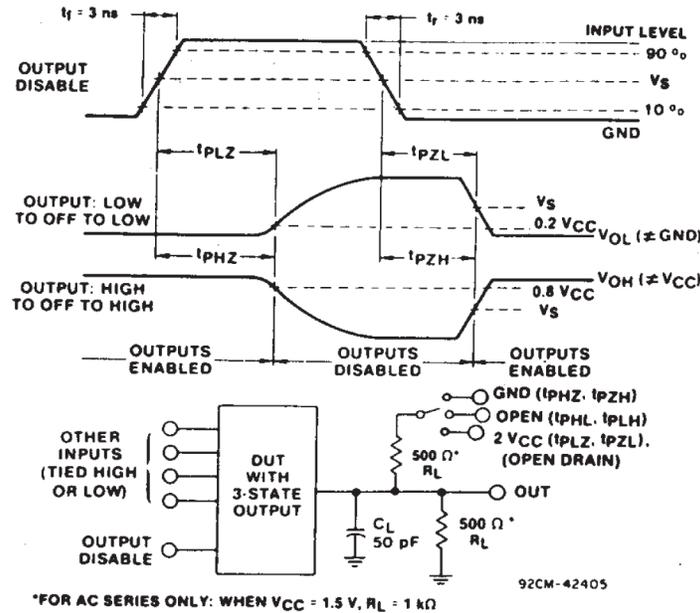
图 5-2. Three-state Propagation Delay Waveforms and Test Circuit.
