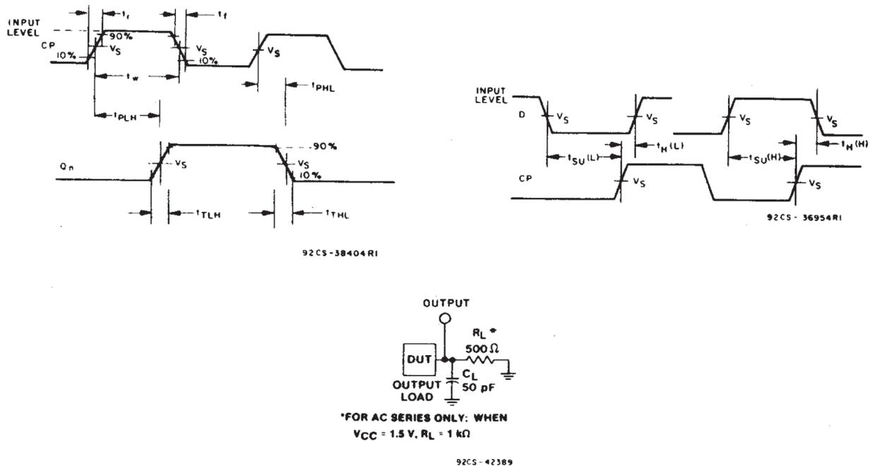
图 5-3. Propagation Delay Times and Test Circuit.
