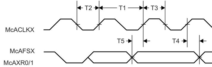
图 7-16. I<sup>2</sup>S Receive Mode Timing Diagram
