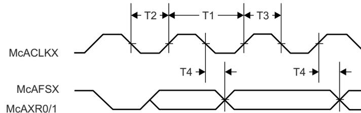
图 7-15. I<sup>2</sup>S Transmit Mode Timing Diagram
