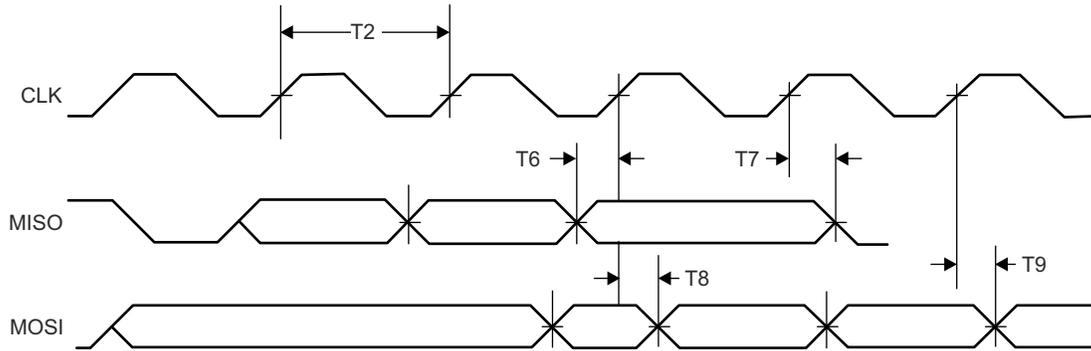
图 7-13. SPI Master Timing Diagram
