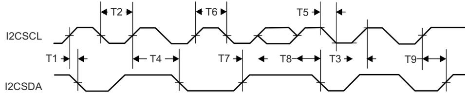
图 7-18. I<sup>2</sup>C Timing Diagram
