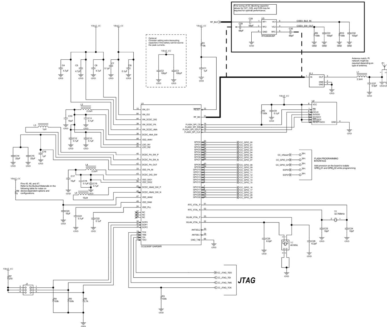
**图 9-5. CC3230x Engine Area and Optional BLE Coexistence**
