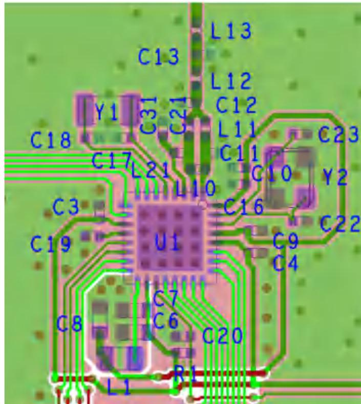
图 10-4. 5 × 5 External Differential (5XD) Layout
