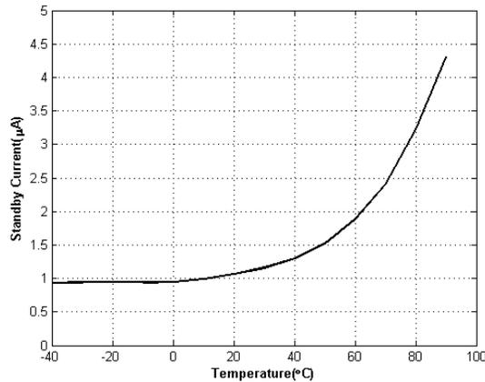
图 8-20. Standby Mode Supply Current vs Temperature
