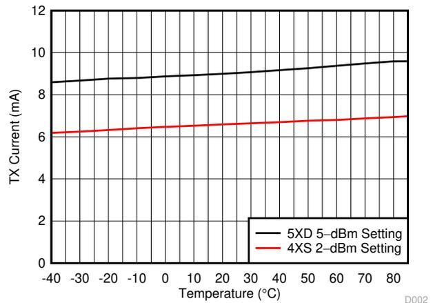
图 8-13. TX Mode Current Consumption vs Temperature
