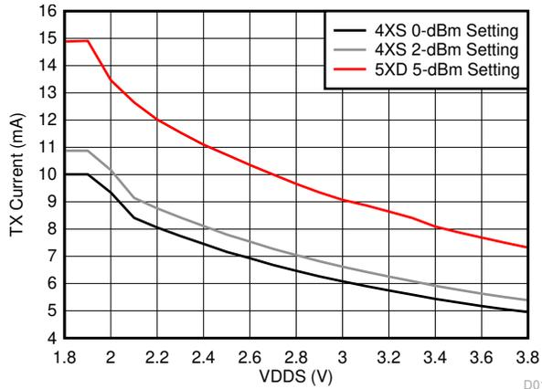
图 8-10. TX Current Consumption vs Supply Voltage (VDD5)
