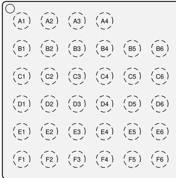
图 7-3. YFV (2.7-mm × 2.7-mm) Pinout, Top View
