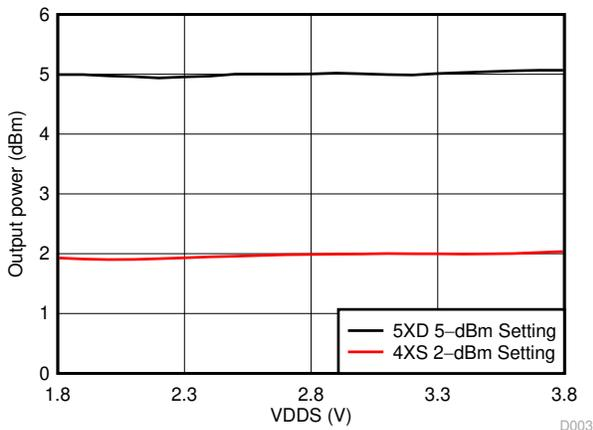
图 8-8. TX Output Power vs Supply Voltage (VDD5)
