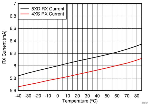
图 8-12. RX Mode Current Consumption vs Temperature
