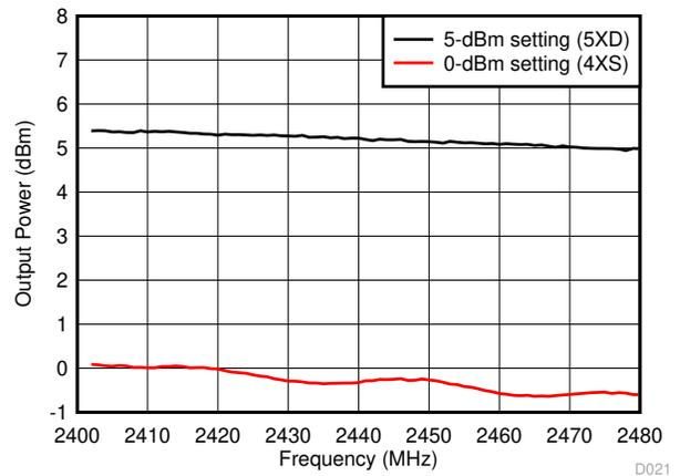
图 8-9. TX Output Power vs Channel Frequency
