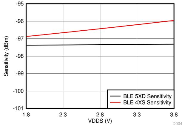
图 8-5. BLE Sensitivity vs Supply Voltage (VDD5)
