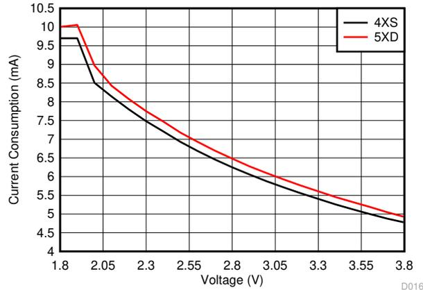
图 8-11. RX Mode Current vs Supply Voltage (VDD5)
