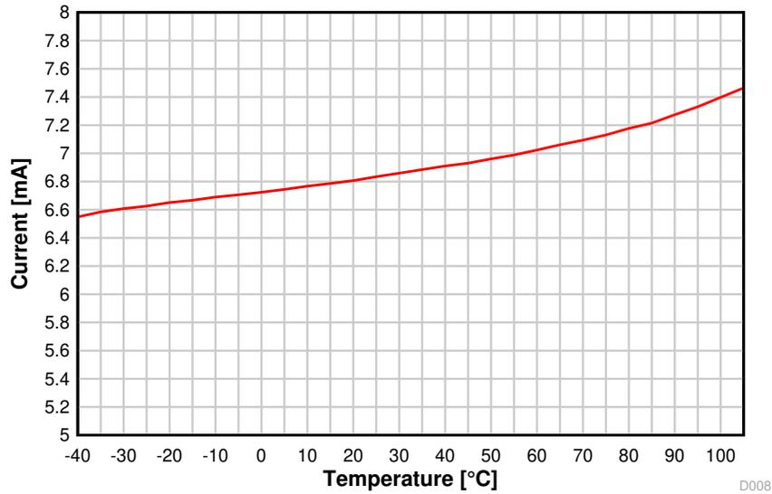
图 8-7. RX Current vs. Temperature (50 kbps, 868.3 MHz)
