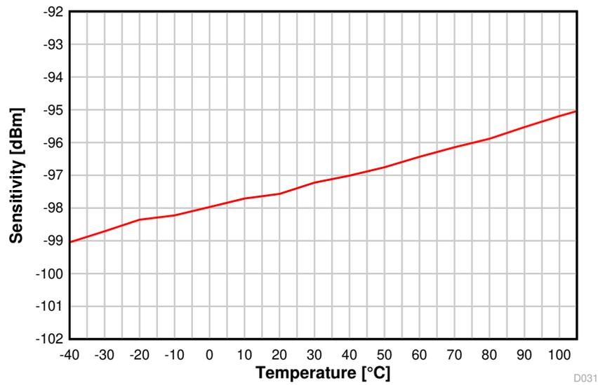
图 8-22. Sensitivity vs. Temperature (BLE 1 Mbps, 2.44 GHz)
