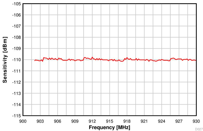
图 8-18. Sensitivity vs. Frequency (50 kbps, 915 MHz)
