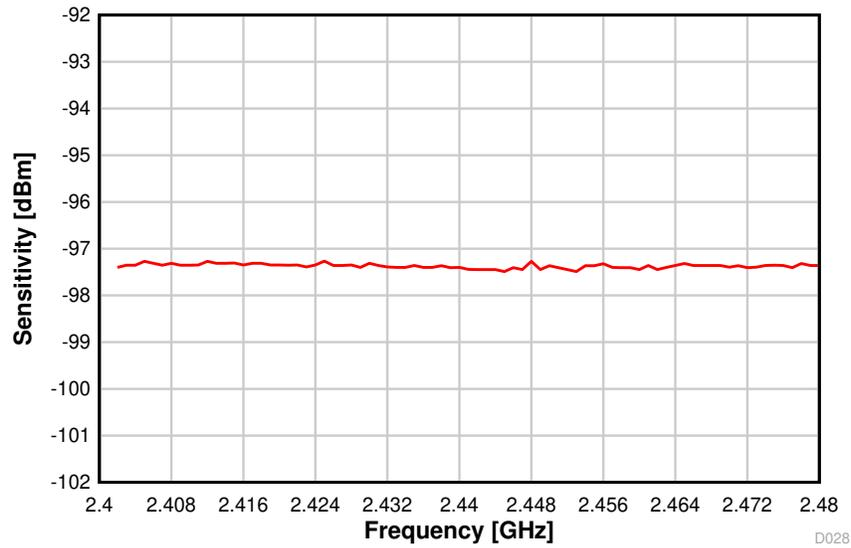
图 8-19. Sensitivity vs. Frequency (BLE 1 Mbps, 2.44 GHz)
