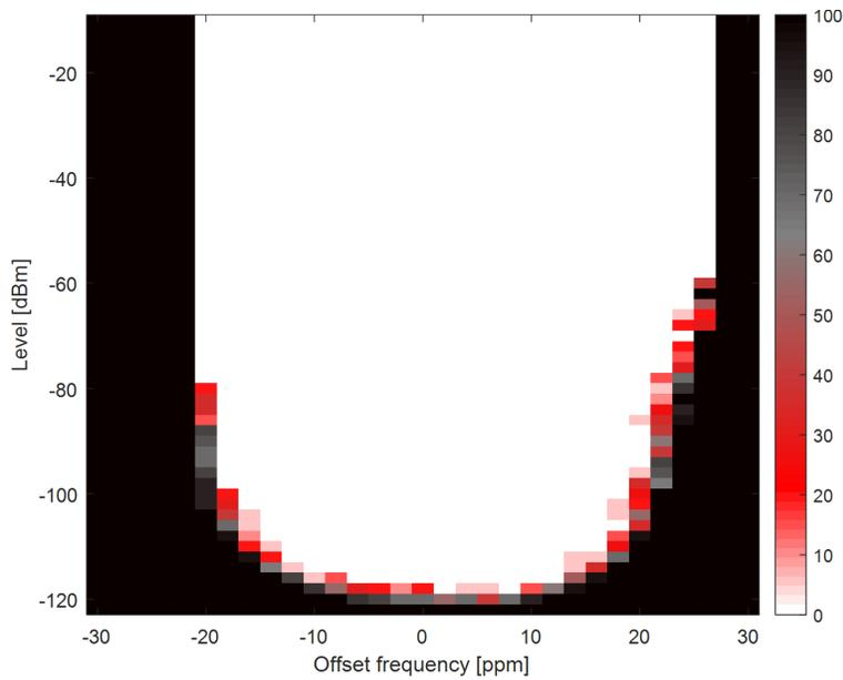
图 8-32. Narrowband, WMBUS N-MODE, 2.4 kbps, 169 MHz
