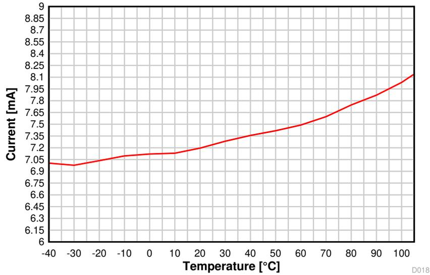
图 8-14. TX Current vs. Temperature (BLE 1 Mbps, 2.44 GHz)
