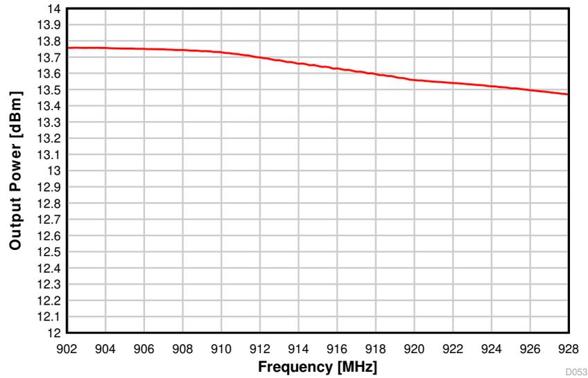
图 8-40. Output Power vs. Frequency (50 kbps, 915 MHz)
