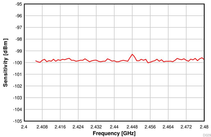
图 8-20. Sensitivity vs. Frequency (250 kbps, 2.44 GHz)
