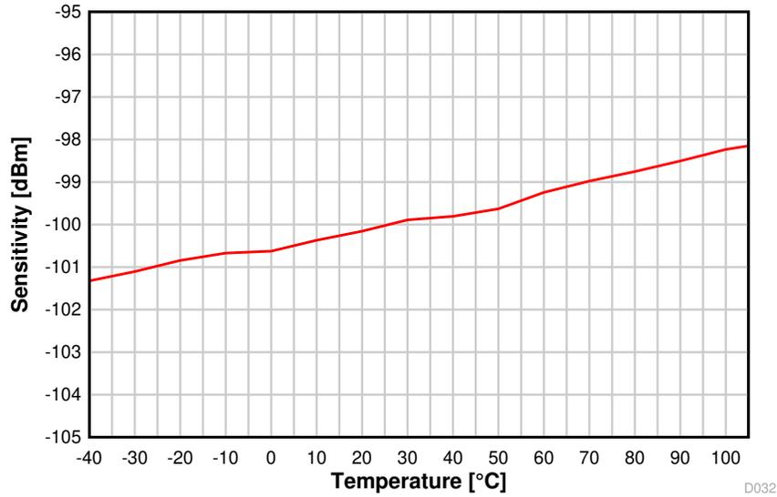
图 8-23. Sensitivity vs. Temperature (250 kbps, 2.44 GHz)
