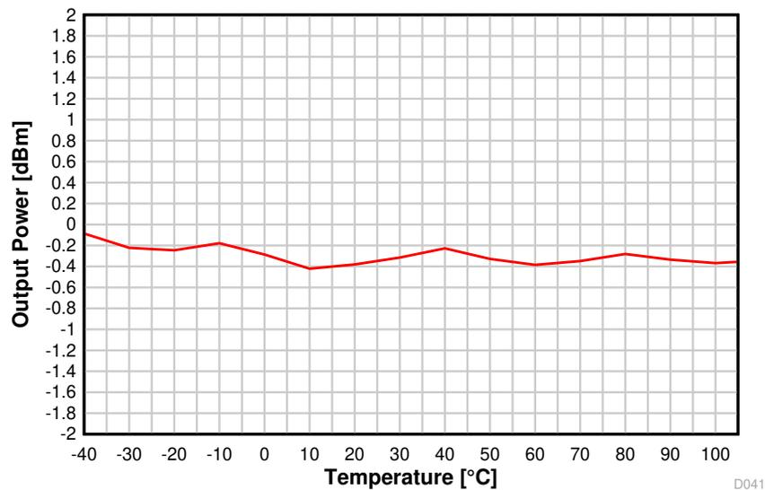
图 8-34. Output Power vs. Temperature (BLE 1 Mbps, 2.44 GHz)
