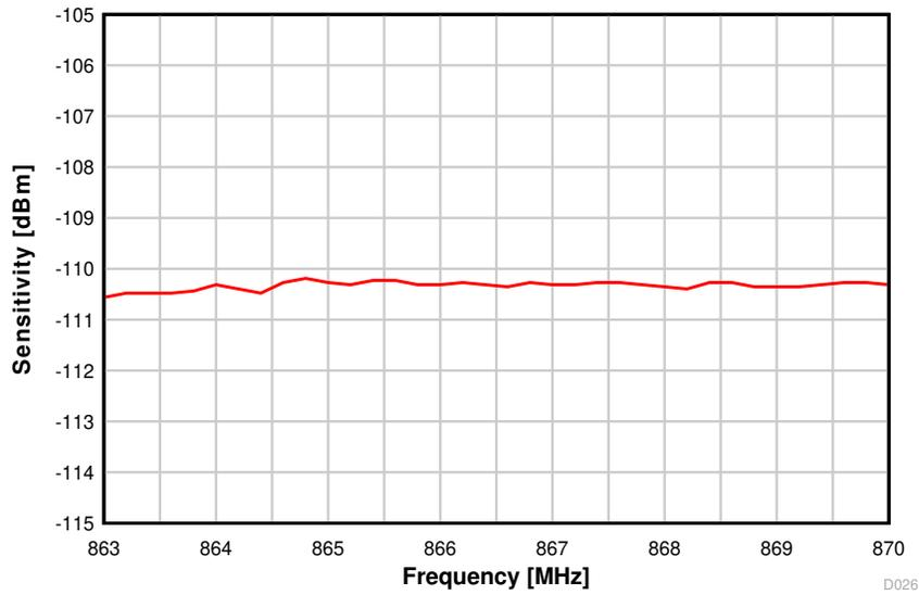
图 8-17. Sensitivity vs. Frequency (50 kbps, 868 MHz)
