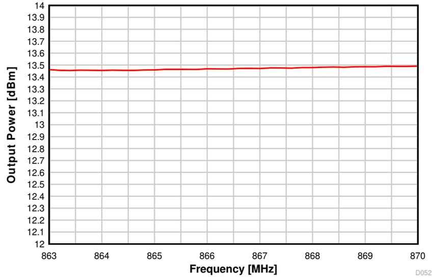
图 8-39. Output Power vs. Frequency (50 kbps, 868 MHz)
