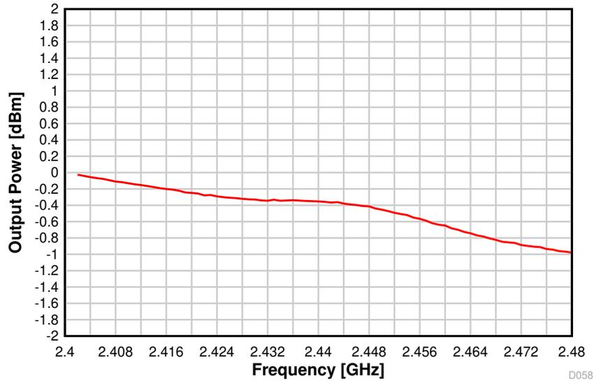
图 8-41. Output Power vs. Frequency (BLE 1 Mbps, 2.44 GHz)
