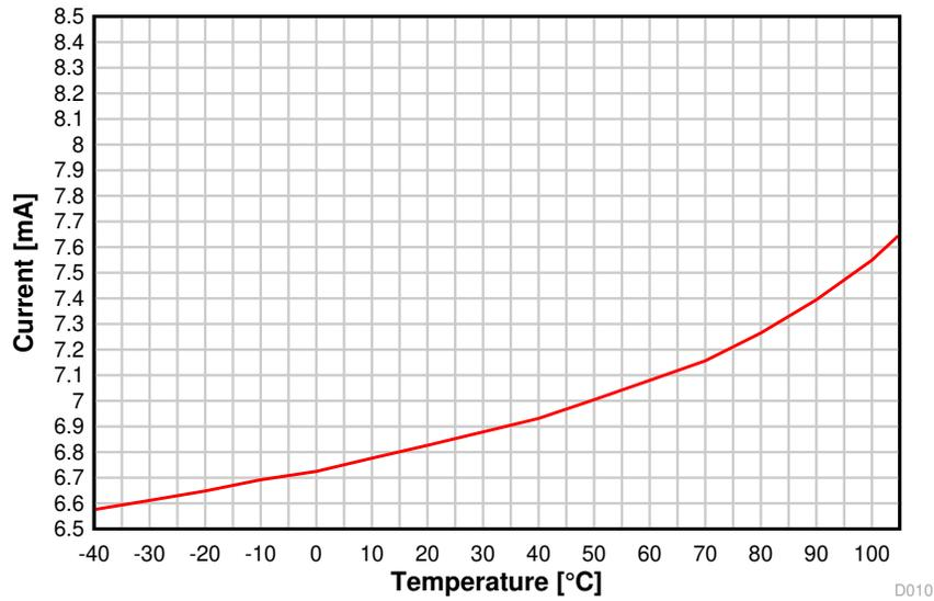
图 8-9. RX Current vs. Temperature (BLE 1 Mbps, 2.44 GHz)
