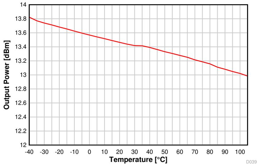
图 8-33. Output Power vs. Temperature (50 kbps, 868.3 MHz)
