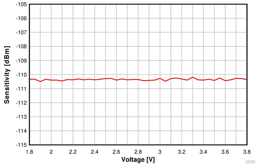
图 8-24. Sensitivity vs. Supply Voltage (VDDS) (50 kbps, 868.3 MHz)
