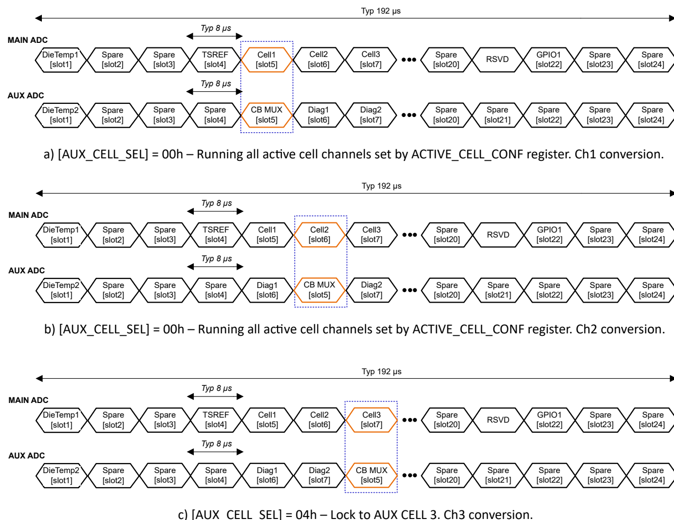
图 8-11. Synchronization Between MAIN and AUX ADC Sampling
