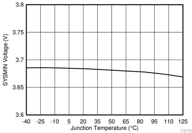
图 7-9. SYSMIN Voltage vs Junction Temperature (VSYS set at 3.5 V)
