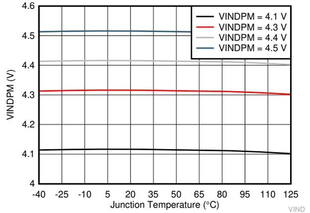
图 7-8. VINDPM vs Junction Temperature
