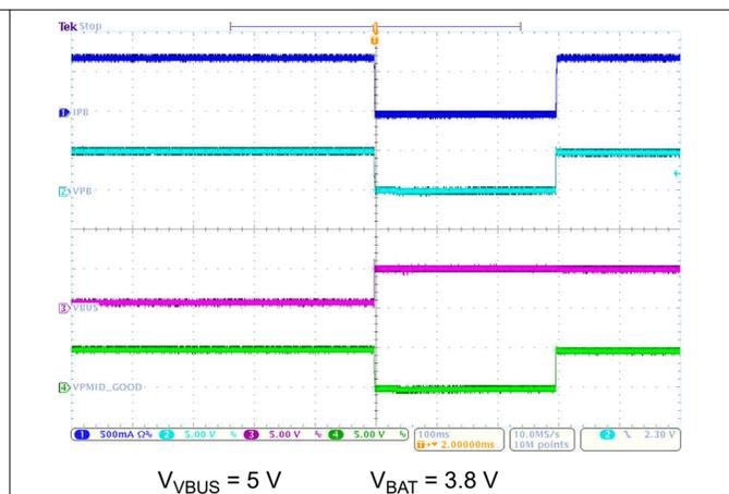
图 9-3. VBUS Plugged In with Boost Mode Enabled
