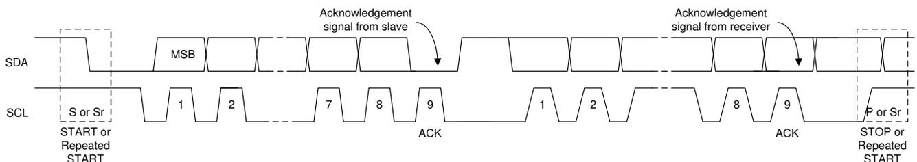
**图 8-9. Data Transfer on the I<sup>2</sup>C Bus**
