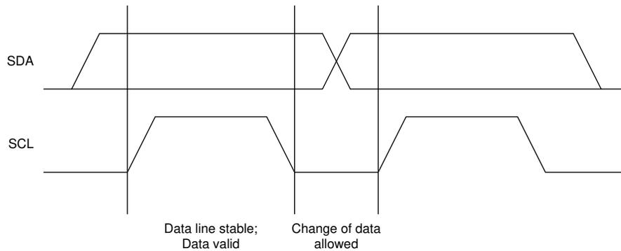
**图 8-7. Bit Transfer on the I<sup>2</sup>C Bus**
