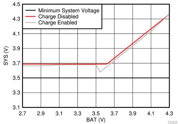
图 8-1. System Voltage vs Battery Voltage
