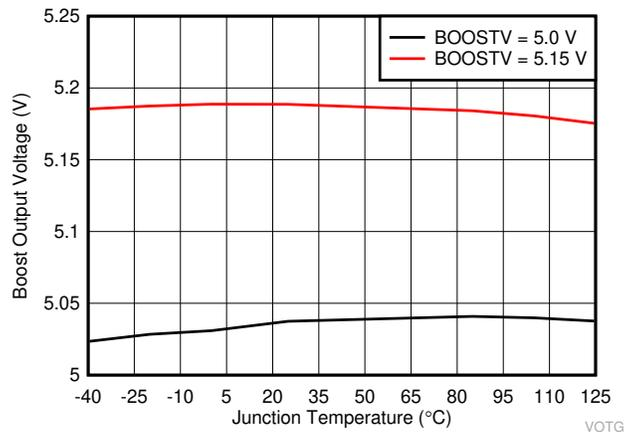
图 7-11. Boost Output Voltage vs Junction Temperature
