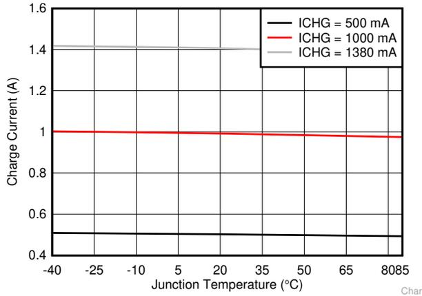
图 7-7. Charge Current vs Junction Temperature
