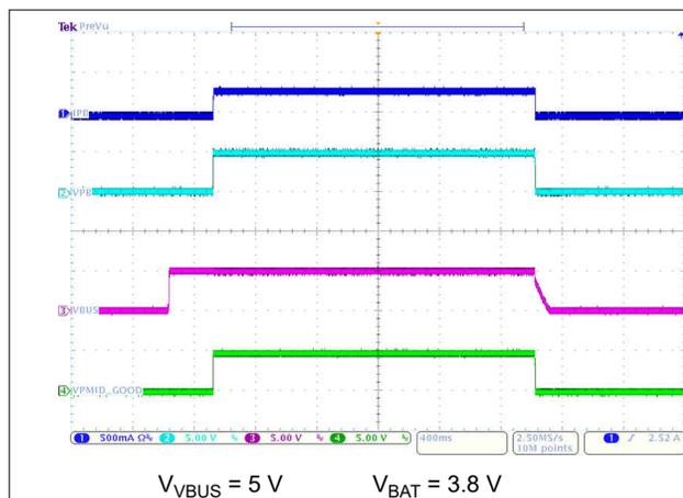
图 9-2. VBUS Plugged In and Unplugged with Boost Mode Disabled
