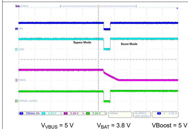
图 9-4. VBUS Unplugged with Boost Mode Enabled
