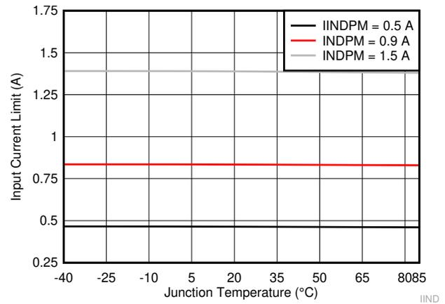
图 7-10. Input Current Limit vs Junction Temperature
