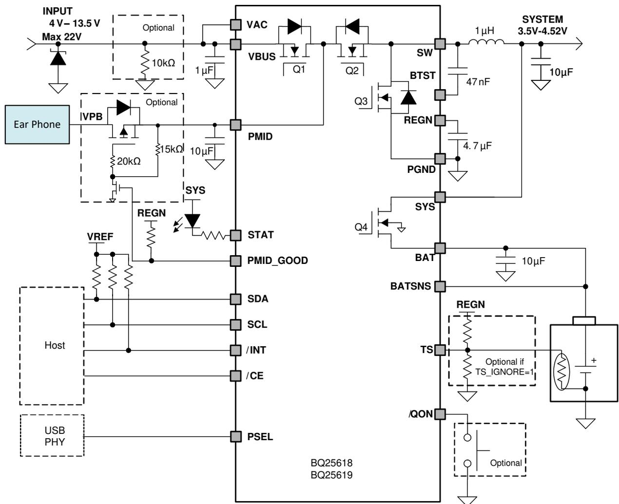
图 9-1. BQ25619 Application Diagram with Optional PMOS
