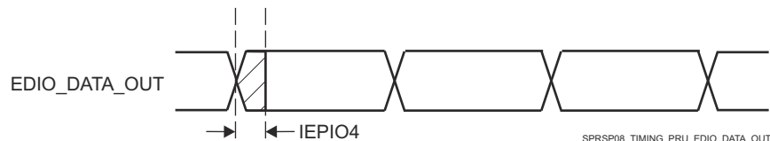
图 6-106. PRU_ICSSG PRU IEP Digital IOs Timing
