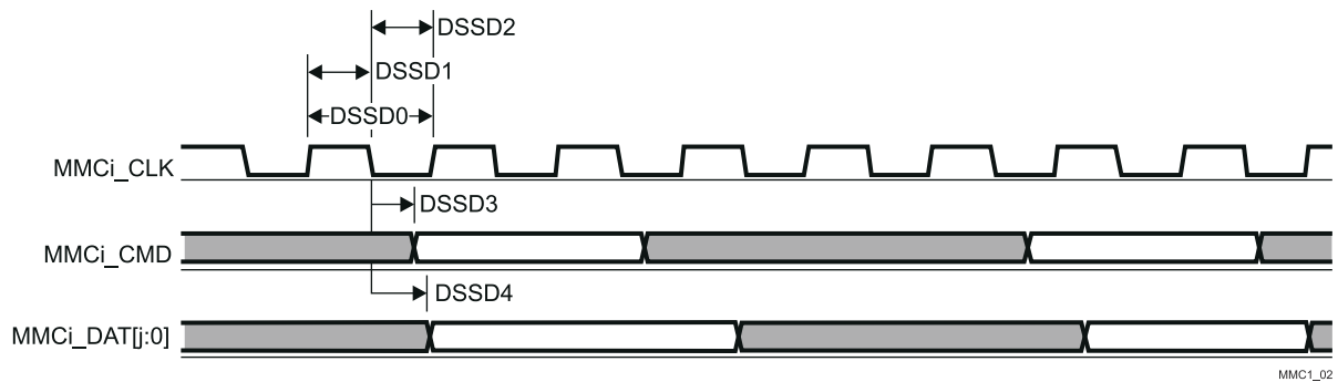
图 6-73. eMMC/SD/SDIO in - Default Speed - Transmitter Mode
