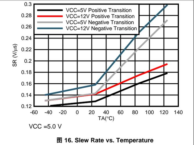
图 16. Slew Rate vs. Temperature
