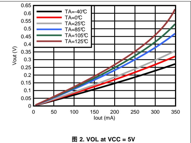
图 2. VOL at VCC = 5 V
