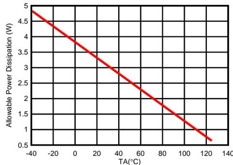
Maximum power dissipation is a function of  $T_{J(max)}$ ,  $\theta_{JA}$ , and  $T_A$ . The maximum allowable power dissipation at any allowable ambient temperature is  $P_D = (T_{J(max)} - T_A)/\theta_{JA}$ . Operating at the absolute maximum  $T_J$  of 150°C can affect reliability.
