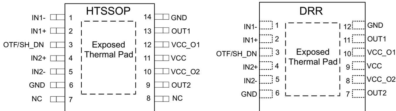
It is recommended to connect the Exposed Pad to ground for best thermal performance. Must not be connected to any other pin than ground. However, it can be left floating.
