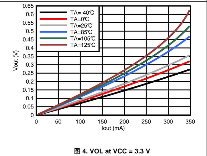
图 4. VOL at VCC = 3.3 V
