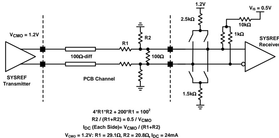
图 51. Example DC Coupling to the SYSREF Input
