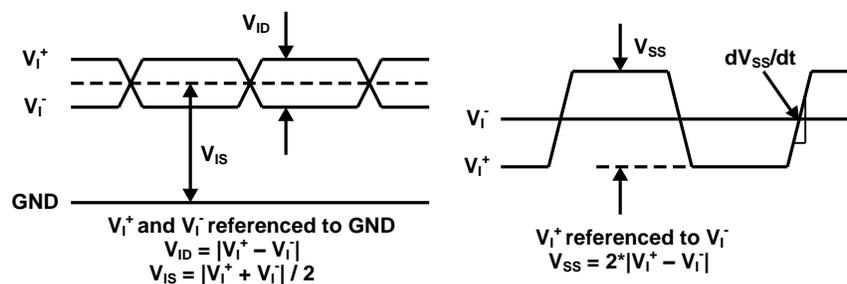
图 1. Electrical Level Diagram for Differential Input Signals
