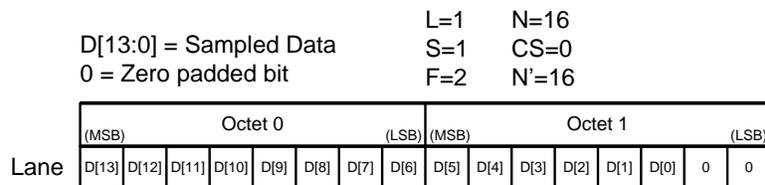
**图 35. Transport Layer Definitions for the Supported-Lane Configurations**
