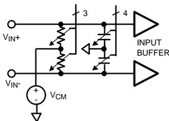
图 32. Simplified Input Differential Balance Correction Circuit
