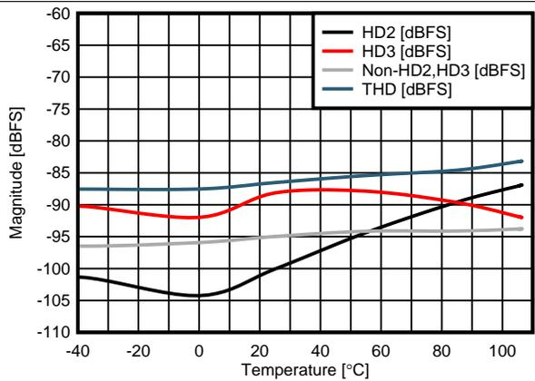
图 23. HD2, HD3, Non-HD2/HD3, THD vs Temperature
