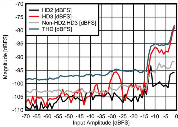
图 21. HD2, HD3, Non-HD2/HD3, THD vs Input Power
