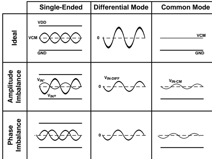
图 39. Differential Signal Waveform and Signal Imbalance
