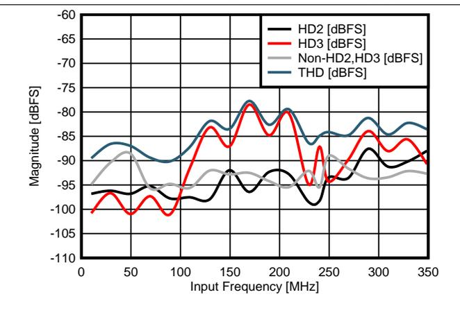
图 20. HD2, HD3, Non-HD2/HD3, THD vs Input Frequency
