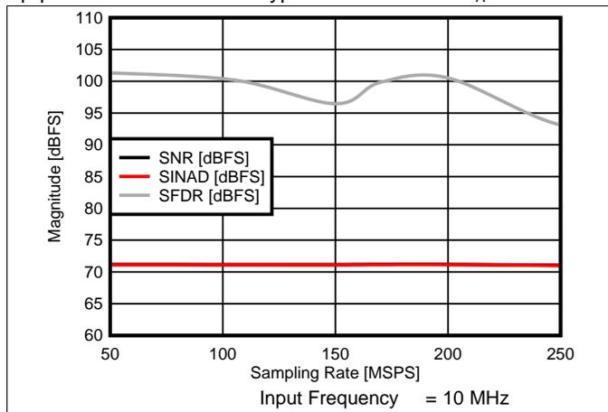
图 15. SNR, SINAD, SFDR vs Sampling Rate
