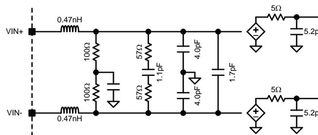
图 40. Simplified Analog Input Network Circuit Model
