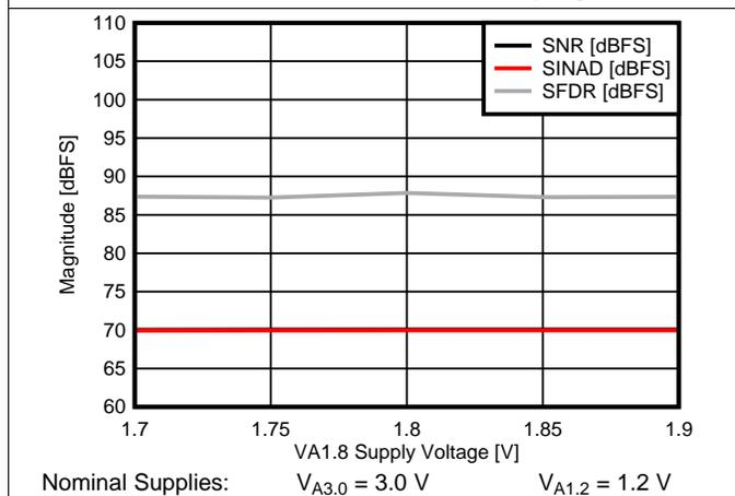
图 17. SNR, SINAD, SFDR vs VA1.8 Supply
