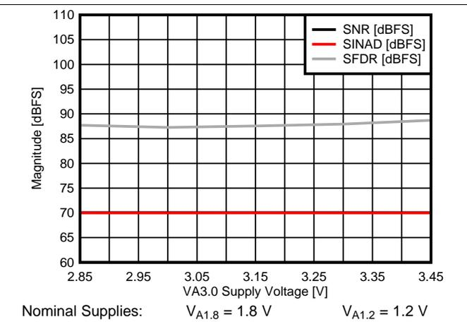
图 16. SNR, SINAD, SFDR vs VA3.0 Supply
