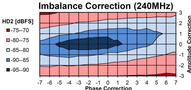
图 33. Gain and Phase Imbalance HD2 Optimization
