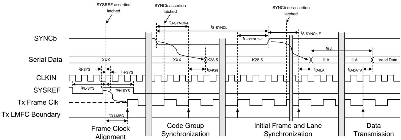
图 8. JESD204B Interface Link Initialization Timing Diagram
