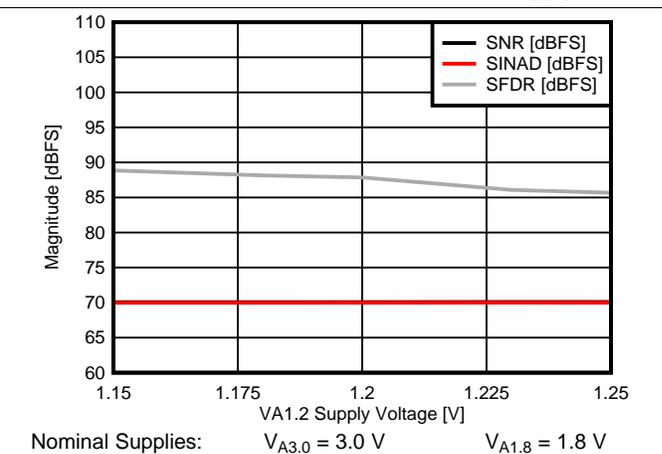
图 18. SNR, SINAD, SFDR vs VA1.2 Supply
