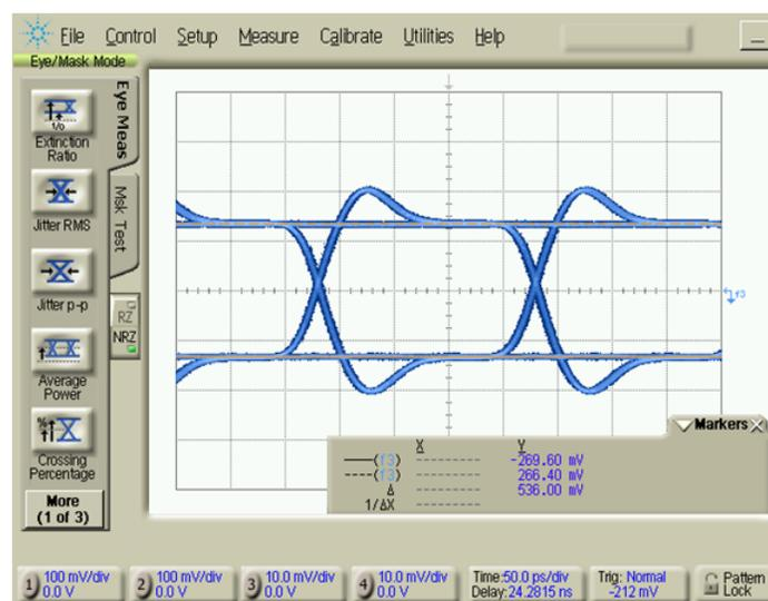
图 34. De-emphasis of the Differential Output Signal
