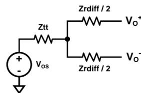
图 4. Electrical Circuit Diagram for Differential Output Signals
