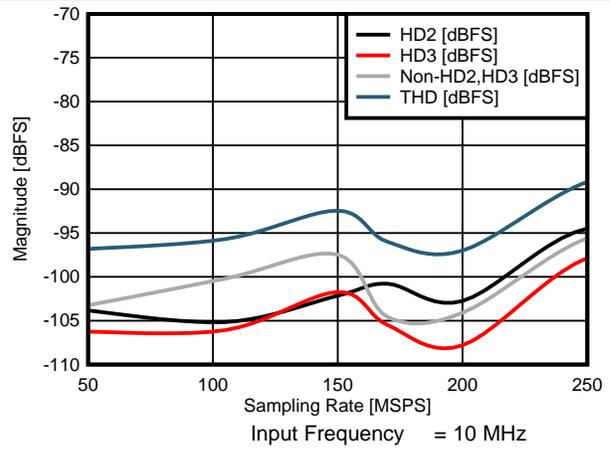
图 22. HD2, HD3, Non-HD2/HD3, THD vs Sampling Rate
