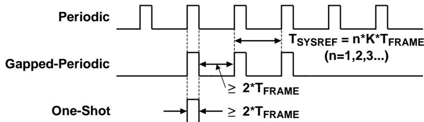
图 52. SYSREF Signal Types (Single-Ended Representations)
