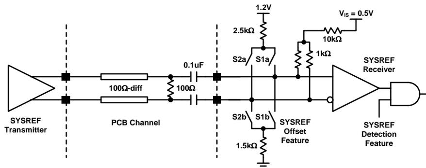
**Figure 50. SYSREF Input Receiver and AC Coupled Interface**
