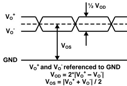
图 3. Electrical Level Diagram for Differential Output Signals
