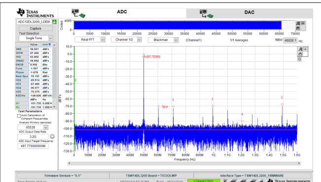
图 8-3. FFT for 497.77-MHz Input Signal in Dual-Channel Mode at 3.2 GSPS
