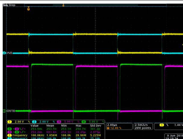
图 9-5. Bench Test Waveform for INA/B and OUTA/B
