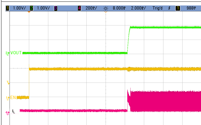
图 9-17. Startup Into 100 mA Electronic Load EN Delay + Soft-Start Delay
