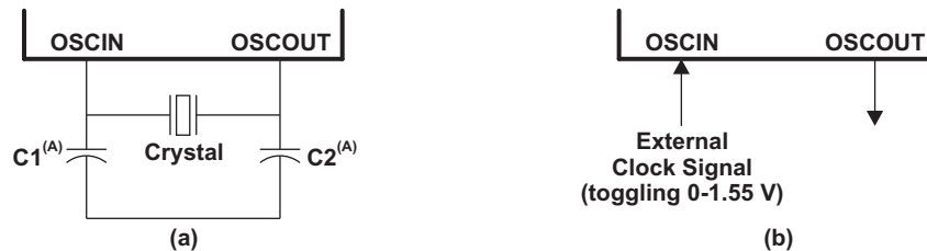
Figure 5-3. Recommended Crystal/Clock Connection
