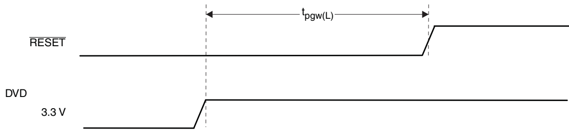
Figure 34. Reset Timing During Power On
