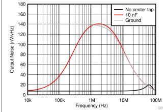
图 9-5. Common-Mode Output Noise for Differential I/O Design
