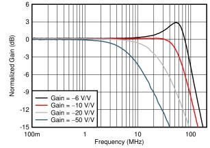
图 7-1. Noninverting Small-Signal Frequency Response vs Gain
