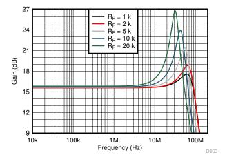
图 8-3. Frequency Response With Various Feedback Resistor Values
