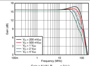
图 7-3. Noninverting Large-Signal Bandwidth vs VOPP
