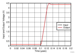
图 8-11. Unipolar Input to Level Shifted Output Step Response
