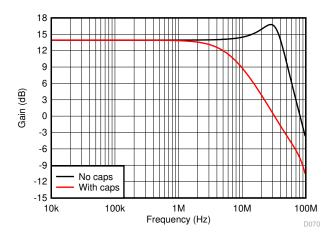
图 8-5. Inverting Response With and Without Compensation
