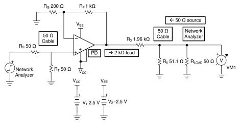
图 9-1. Noninverting Characterization Circuit
