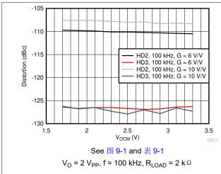
图 7-17. Noninverting Distortion vs Output Common-Mode Voltage
