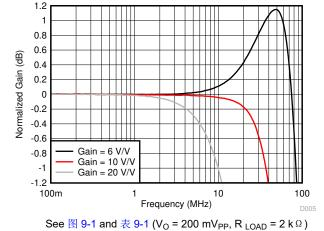
图 7-5. Noninverting Response Flatness vs Gain
