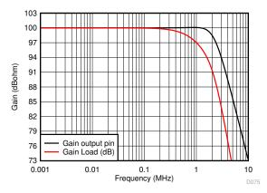
图 9-8. Small-Signal Response for 100-k Ω Transimpedance Gain
