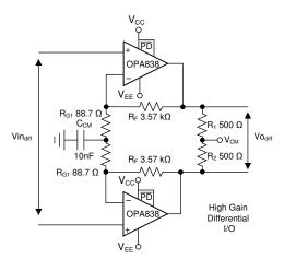
图 9-4. High-Gain Differential I/O Stage
