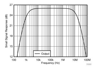
图 8-13. Inverting Single-Supply Response With AC-Coupled Input
