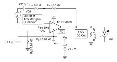
图 8-12. Single-Supply Inverting Gain Stage With AC-Coupled Input
