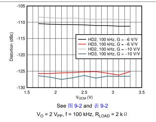
图 7-18. Inverting Distortion vs Output Common-Mode Voltage
