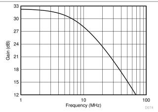
图 9-6. Differential Small-Signal Frequency Response
