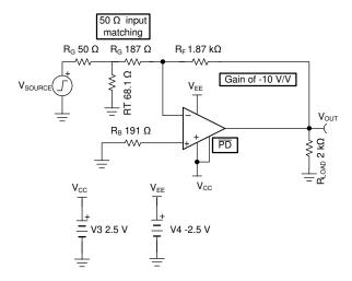
图 9-2. Inverting With Input Impedance Matching
