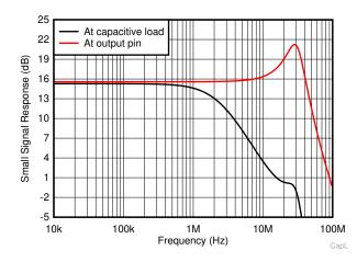
图 8-7. Frequency Response to Output Pin and Capacitive Load
