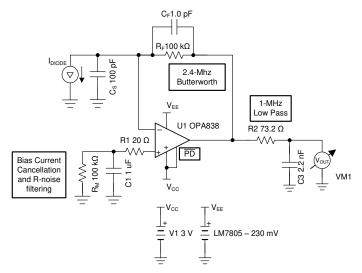
图 9-7. 100-k Ω Wide Bandwidth Transimpedance Design
