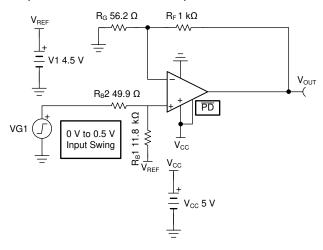
图 8-10. DC-Coupled, Single-Supply, Noninverting Interface With Output Level Shift
