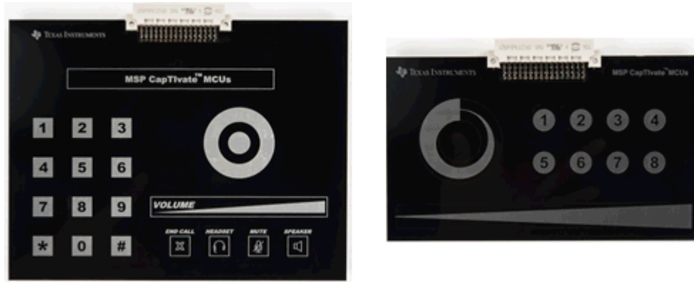
Figure 7-6. CAPTIVATE-PHONE and CAPTIVATE-BSWP Panels
