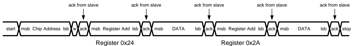
Figure 74. Example Multi-Byte Command Sequencing
