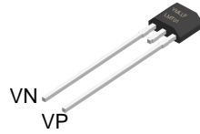
LPG Package 2-Pin TO-92 Top View
