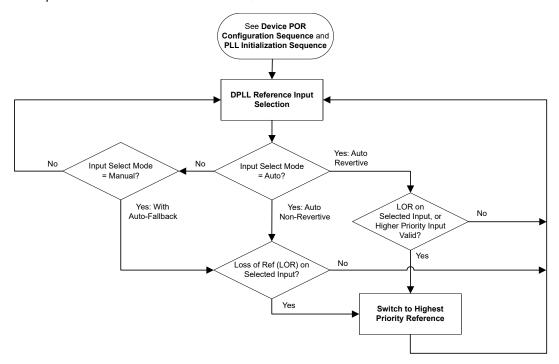
图 8-14. DPLL Reference Input Selection Flowchart
