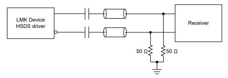
图 8-26. AC-Coupled HSDS Output Termination Method 2
