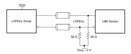
图 8-11. DC-Coupled LVPECL to Reference (INx)
