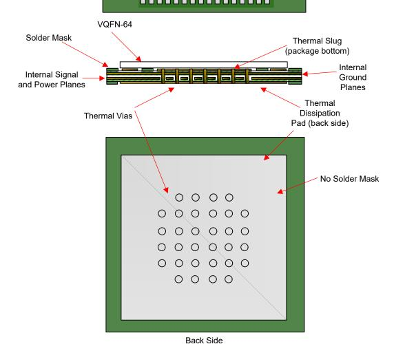
图 9-20. General PCB Ground Layout for Thermal Reliability (8+ Layers Recommended)
