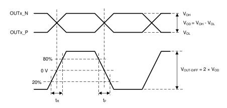
图 6-5. Differential Output Voltage and Rise/Fall Time
