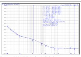
Jitter = 65 fs RMS (12 kHz to 20 MHz)  $f_{APLL3}$  =2500 MHz (APLL3 post-div = 5, Channel-div = 4)
