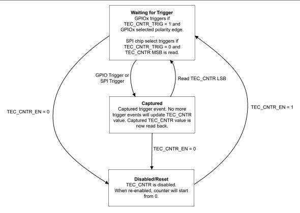
图 8-31. State Diagram of TEC
