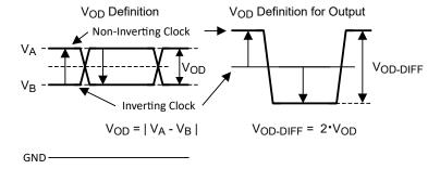
图 7-2. Two Different Definitions for Differential Output Signals
