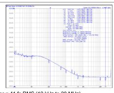
Jitter = 41 fs RMS (12 kHz to 20 MHz) f<sub>APLL3</sub> =2500 MHz (APLL3 post-divider = 8)
