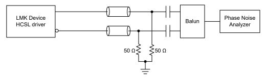
图 7-8. HCSL Output Time Domain Test Configuration
