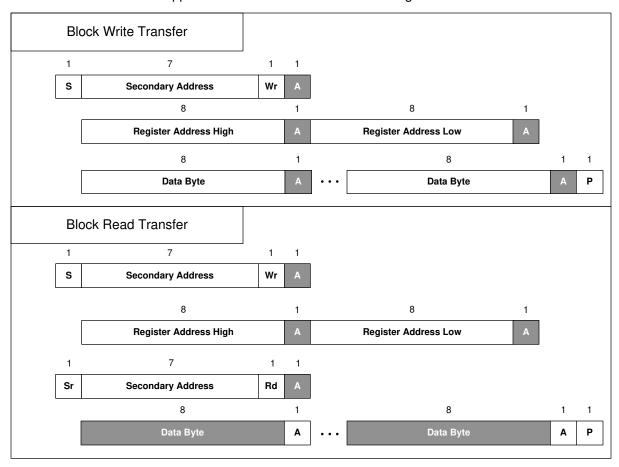
图 8-41. I<sup>2</sup>C Block Register Transfers
