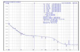
图 9-13. 122.88 MHz Output Phase Noise (APLL2)
