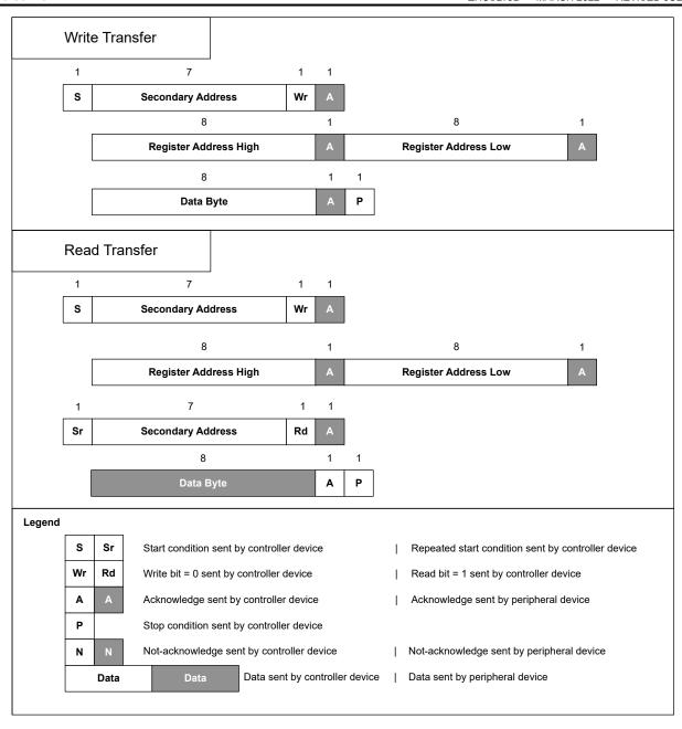
图 8-40. I<sup>2</sup>C Byte Write and Read Transfers
