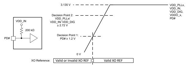
图 9-1. Recommendation for Power Up From a Single-Supply Rail
