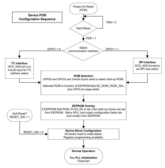
图 8-35. Device POR Configuration Sequence
