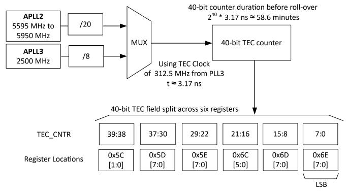
图 8-30. TEC Clock and Counter
