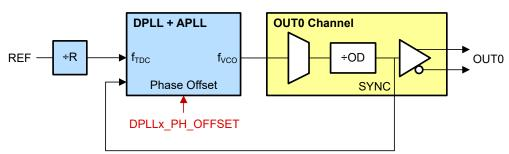
图 8-29. DPLL ZDM Synchronization Between Reference Input and OUT0
