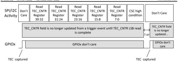
图 8-34. TEC Captured Using GPIO
