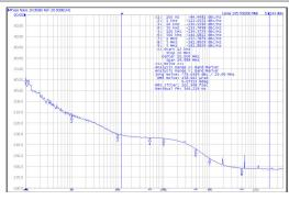
Jitter = 102 fs RMS (12 kHz to 20 MHz)
