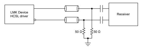
图 8-28. AC-Coupled HCSL Output Termination
