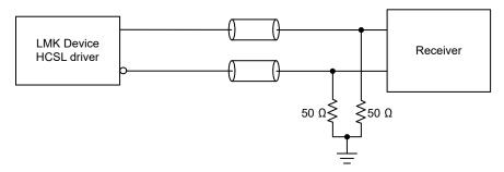
图 8-27. DC-Coupled HCSL Output Termination
