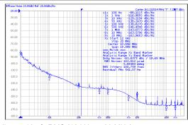
Jitter = 105 fs RMS (12 kHz to 20 MHz)  $f_{APLL2}$  = 5800.78125 MHz
