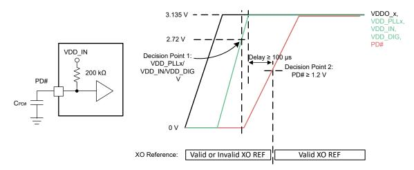
图 9-2. Recommendation for Power Up From Split-Supply Rails
