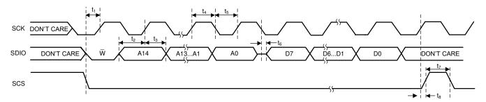
图 6-3. SPI 3-Wire Read Timing Diagram
