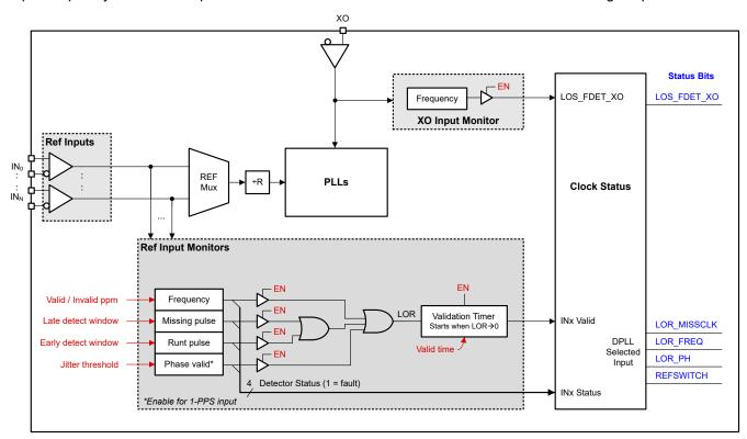
图 8-15. Clock Monitors for Reference and XO Inputs
