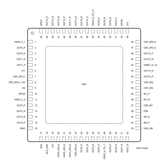
图 5-1. LMK5B33216 RGC Package 64-Pin VQFN Top View
