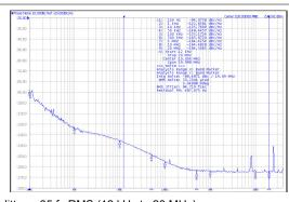
Jitter = 85 fs RMS (12 kHz to 20 MHz)  $f_{APLL3}$  =2500 MHz (APLL3 post-div = 5, Channel-div = 5)
