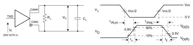
A. The input pulse is supplied by a generator having the following characteristics: PRR  $\le$  125 kHz, 50% duty cycle, tr  $\le$  6 ns, tf  $\le$  6 ns, ZO = 50  $\Omega$ .
