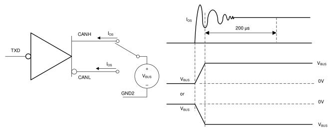
图 7-8. Driver Short-Circuit Current Test Circuit and Waveforms
