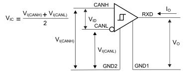
图 7-4. Receiver Voltage and Current Definitions
