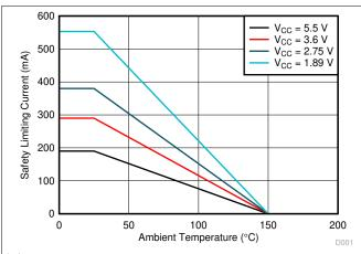
图 6-1. Thermal Derating Curve for Limiting Current per VDE for 8-D Package
