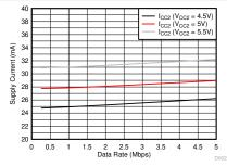
图 6-4. Side 2 Supply Current vs Datarate
