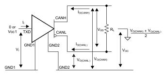
图 7-1. Driver Voltage, Current and Test Definitions
