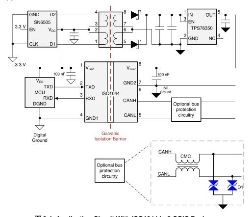
图 9-1. Application Circuit With ISO1044 in 8-SOIC Package
