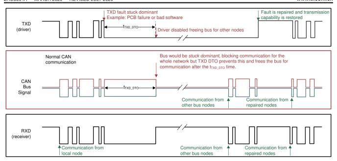
图 8-3. Example Timing Diagram for TXD DTO
