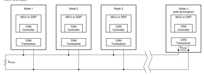
图 9-2. Typical CAN Bus
