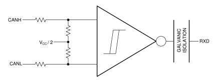
图 8-2. Simplified Recessive Common Mode Bias and Receiver
