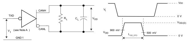
A. The input pulse is supplied by a generator having the following characteristics:  $t_r \leqslant 6$  ns,  $t_f \leqslant 6$  ns,
