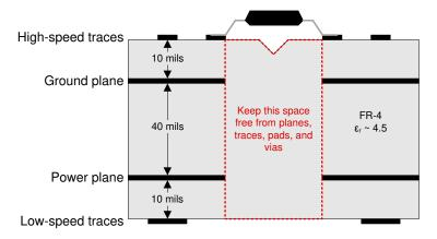
图 11-1. Recommended Layer Stack
