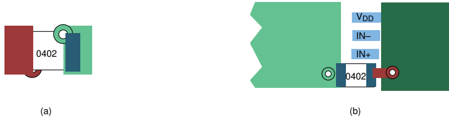
图 11-7. Typical Decoupling Capacitor Layouts
