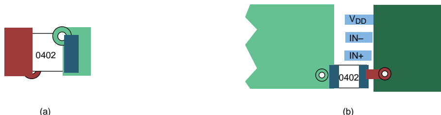
Figure 22. Typical Decoupling Capacitor Layouts
