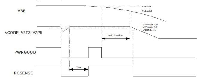
Figure 3. Power Down Sequencing Timing Diagram
