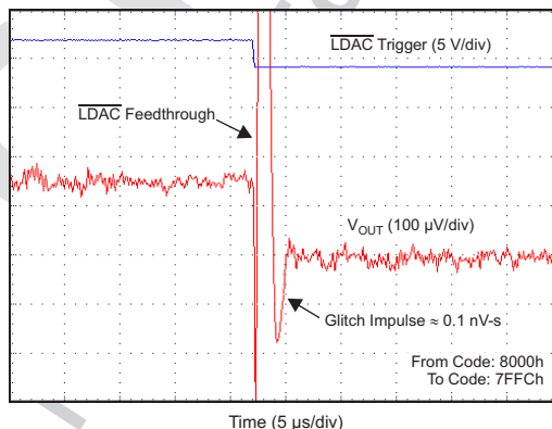
图 80. Glitch Impulse Falling Edge, 1-LSB Step
