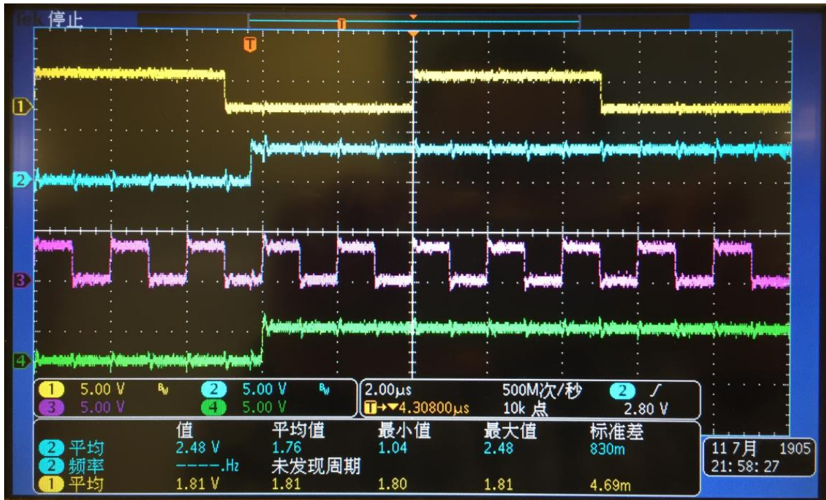
Figure 10. 零脉宽即 0%高电平切换到全脉宽即 100%高电平输出
