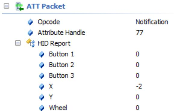
**Figure 4-6. Parsed Mouse Notification Payload**
