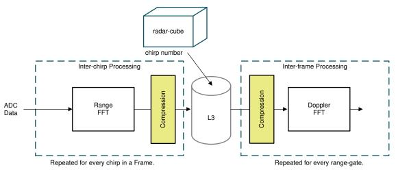
Figure 3. Standard Radar Processing Flow
