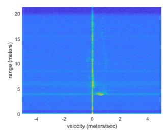
Figure 9. The Range-Doppler Image Resulting From 33% Compression Across Antennas
