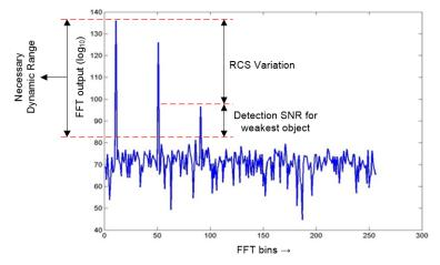
Figure 5. Dynamic Range Necessary for Proper Radar Operation
