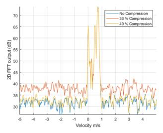
Figure 10. Range-Gate Picture for Compression Across Antennas
