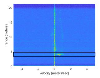
Figure 7. Range-Doppler Image for a 33% Compressed Radar Cube
