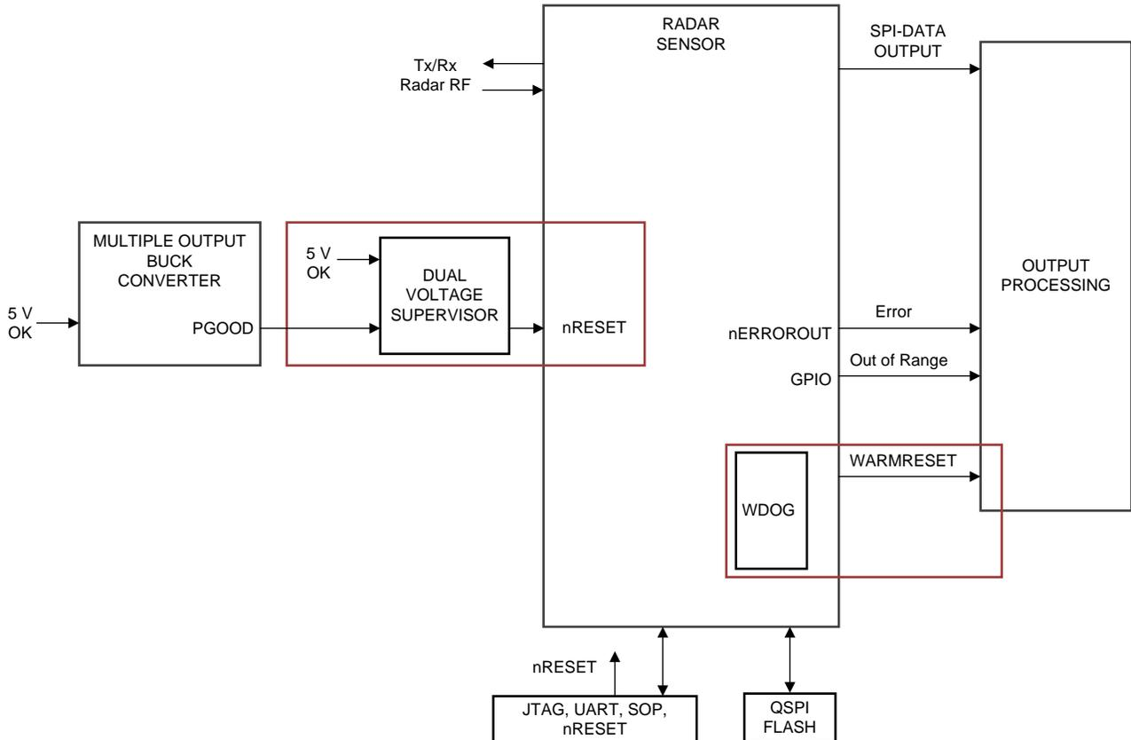
Figure 4. Stand-Alone Radar Sensor – Internal Watchdog Timer (WDOG)
