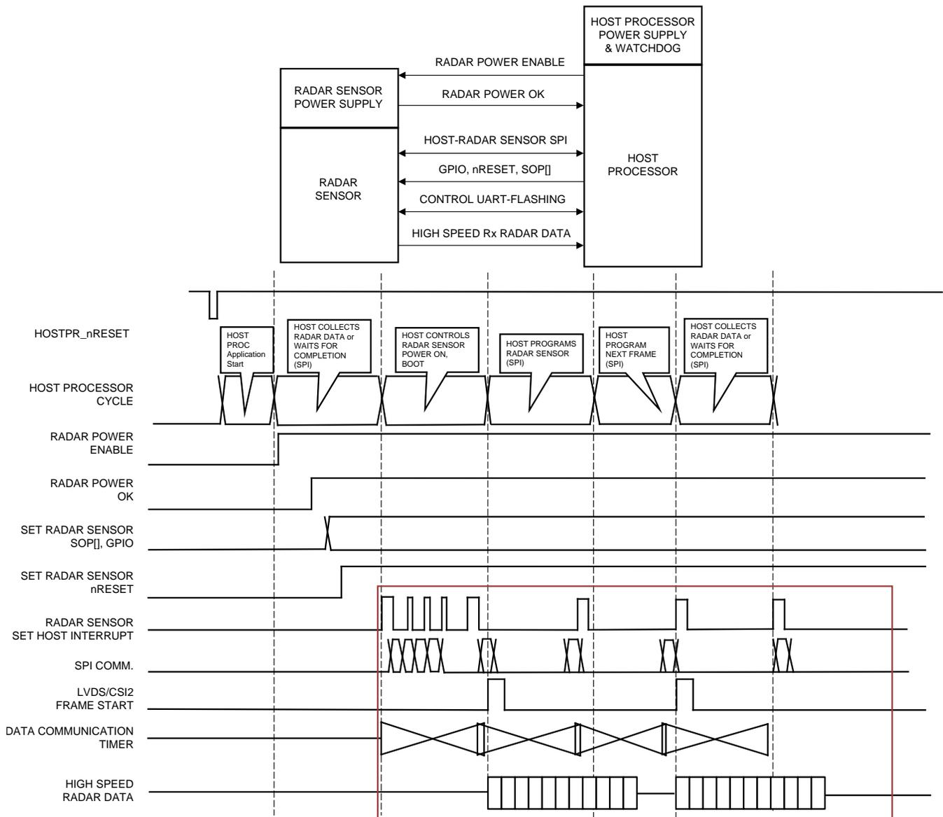
Figure 3. Host Processor Control and Data Communication Timer
