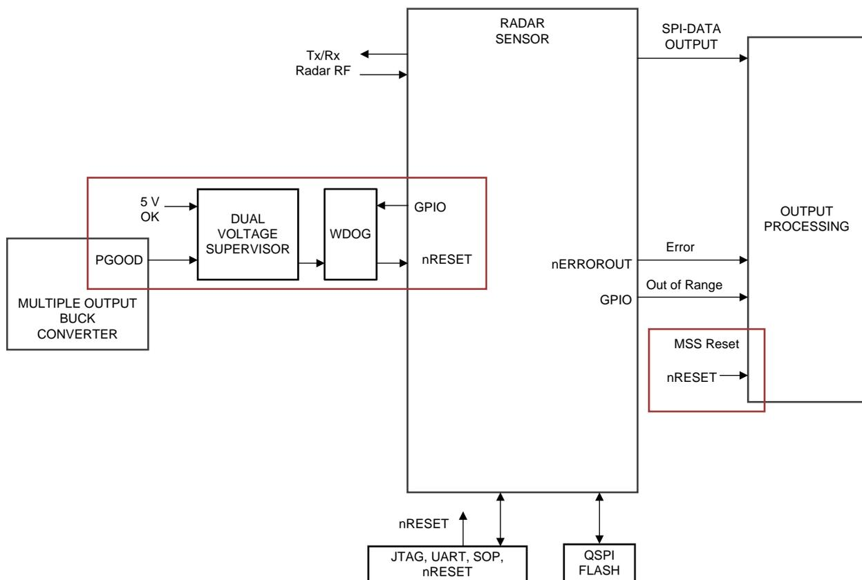
Figure 5. Stand-Alone Radar Sensor – External Watchdog Timer (WDOG)
