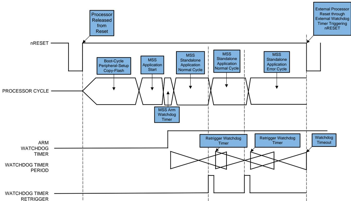
Figure 2. Radar Sensor With External Watchdog Timer
