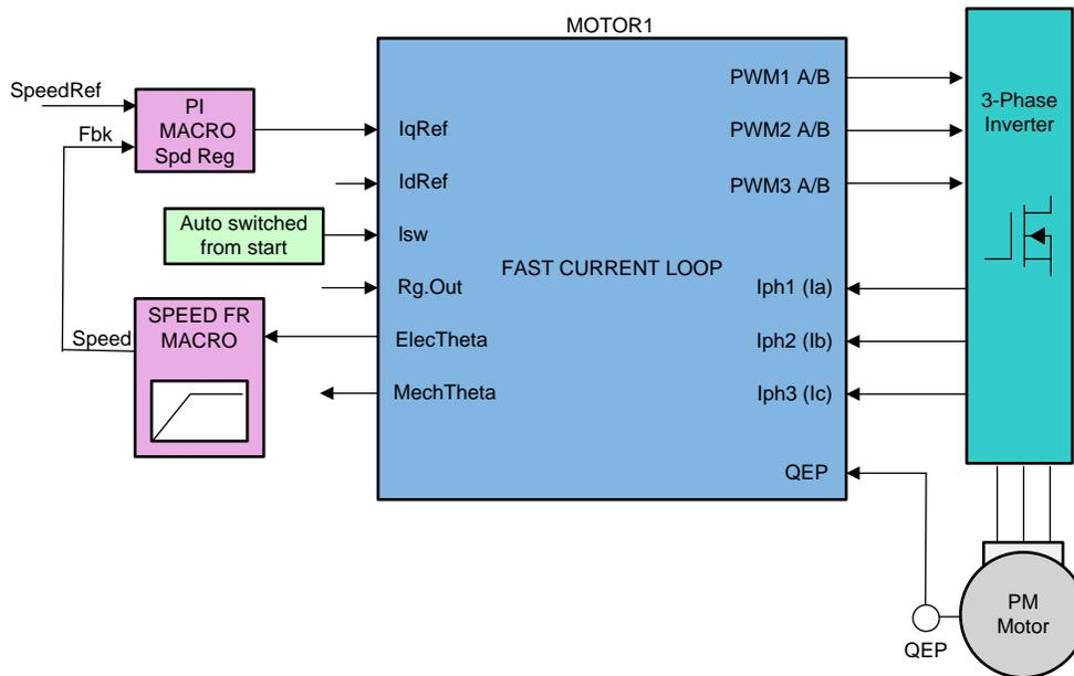
Figure 9. Level 4 Incremental System Build Block Diagram
