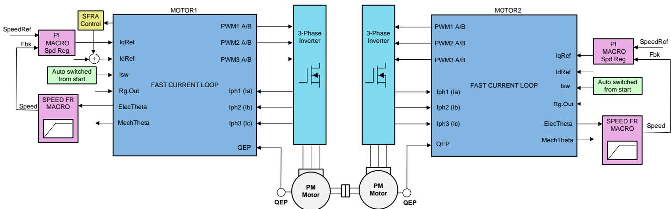
Figure 10. Level 6 Incremental System Build Block Diagram
