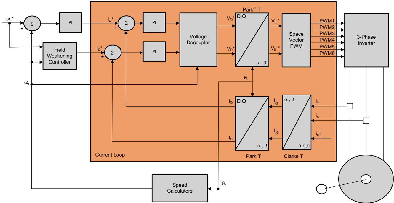
**Figure 1. Speed Control Block Diagram of AC Motors**
