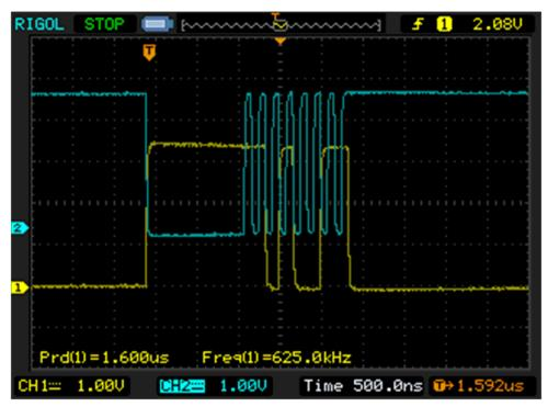
Figure 3-15. Shift Right Once All Other Data and Clock Generation - CPOL=1, CPHA=0
