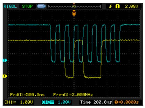
Figure 3-11. Rotate Right Once - CPOL=1, CPHA=1
