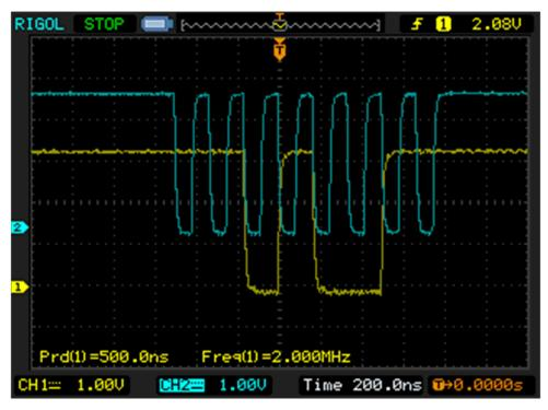
Figure 3-12. Rotate Right Once - CPOL=1, CPHA=0
