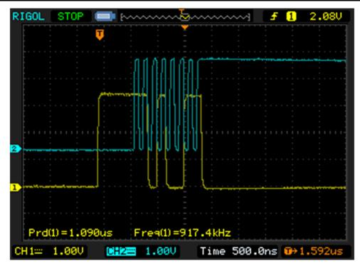
Figure 3-14. Shift Right Once First Data and Clock Generation - CPOL=1, CPHA=0
