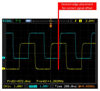
Figure 3-4. Generated Signal Offset - Shift by 3
