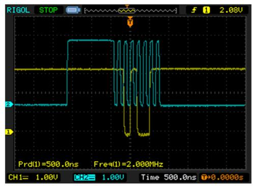
Figure 3-18. Shift Right Once All Other Data and Clock Generation - CPOL=0, CPHA=0
