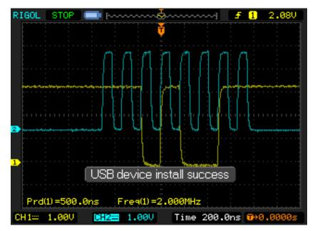
Figure 3-10. Rotate Right Once - CPOL=0, CPHA=0
