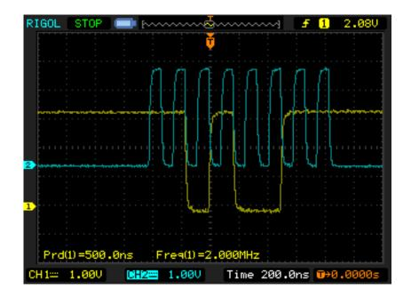
Figure 3-8. Rotate Right Once - CPOL=0, CPHA=1
