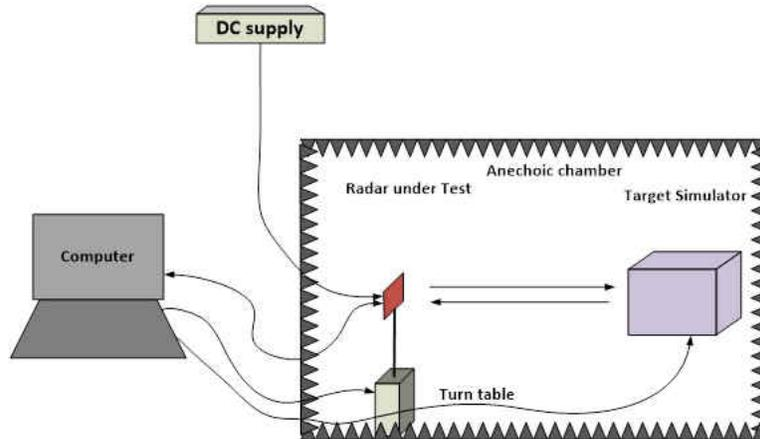
Figure 3-1. Hardware for Radar Testing using Target Simulator
