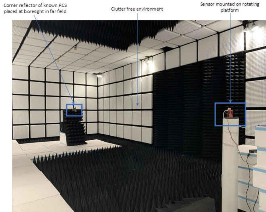
**Figure 2-1. Example Test Environment**
