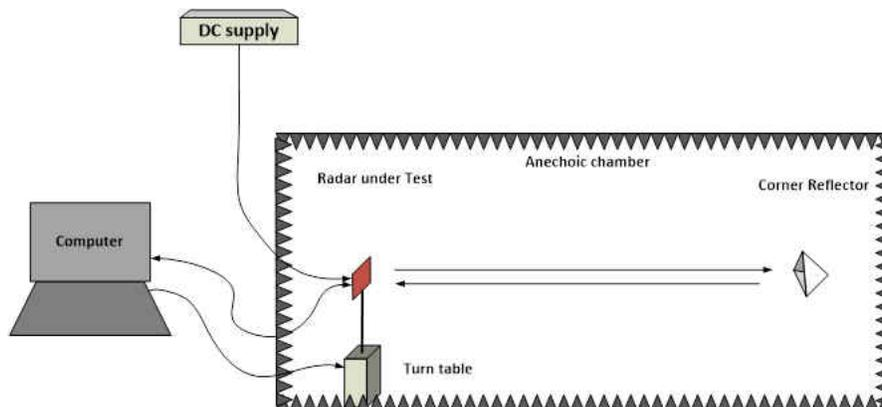
**Figure 2-2. Hardware for Basic Radar Testing**
