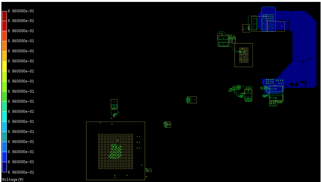
Figure 7. Voltage Map - PMIC_VDD_CTRL
