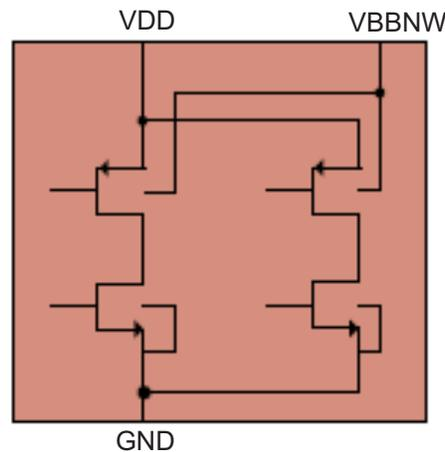
**Figure 4. VDD and VBBNW Supply to Device Transistors**
