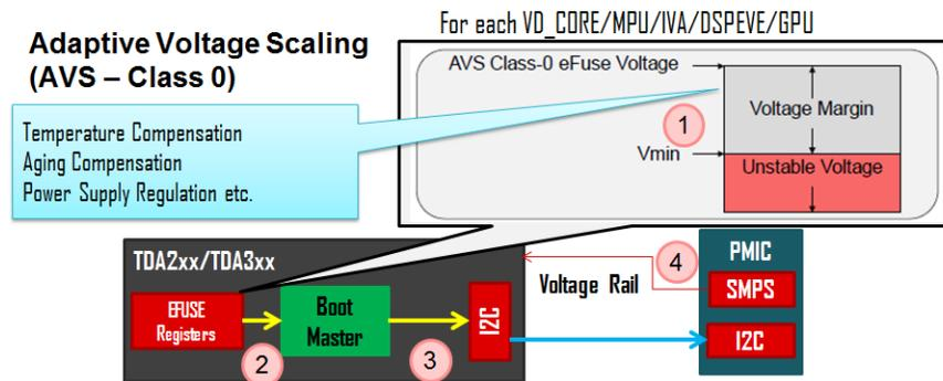
Figure 3. AVS Class 0 Voltage Scaling Mechanism
