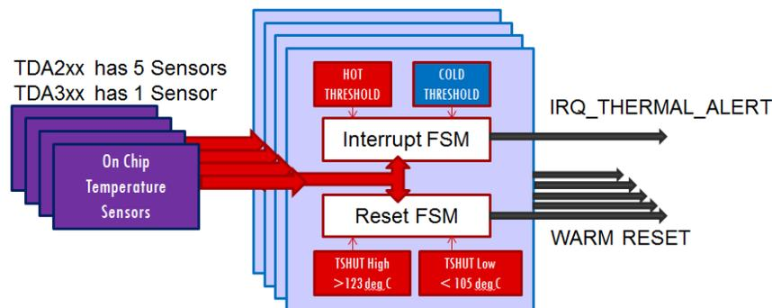
Figure 19. Functional Block Diagram of the Thermal Sensors
