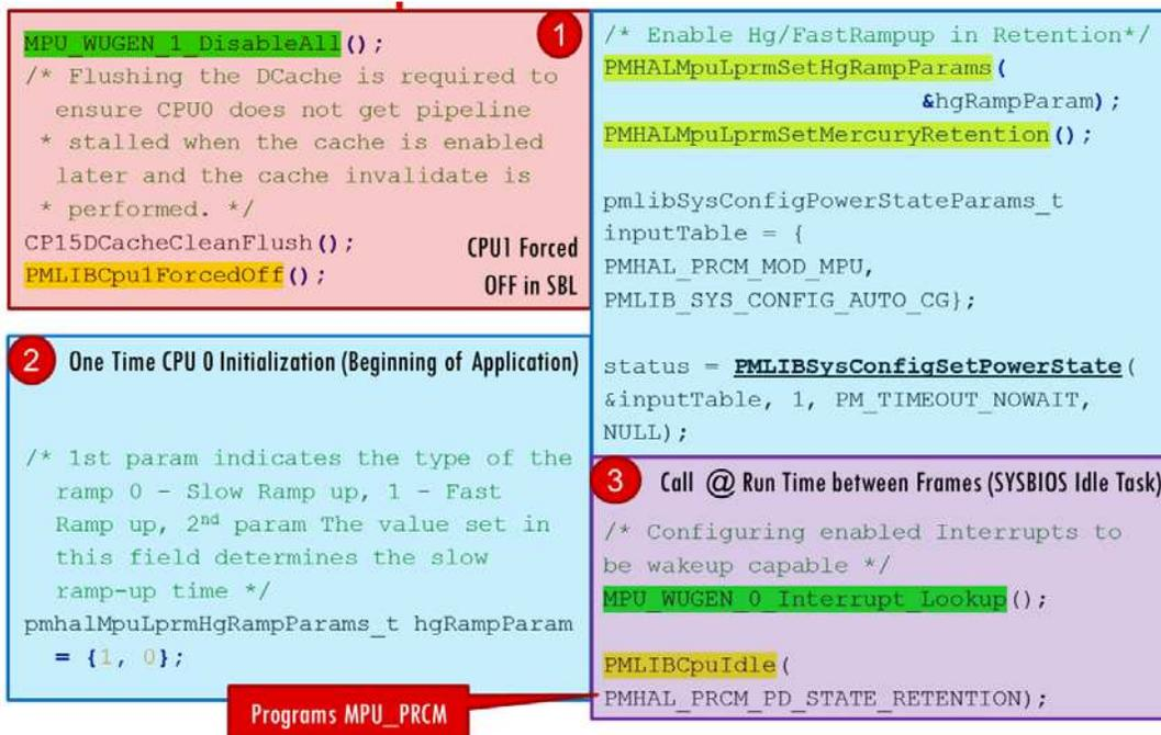
**Figure 12. MPU Recommended Dynamic Power Management Software Flow**
