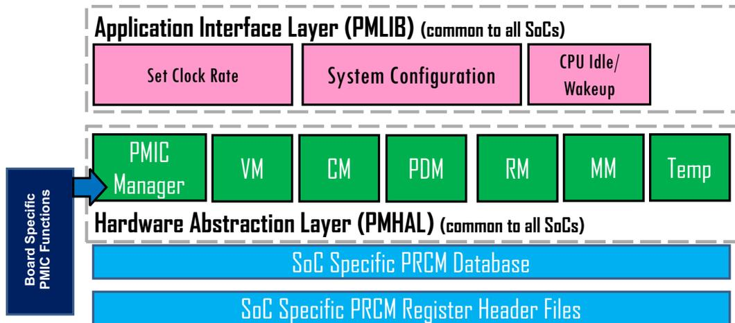
Figure 2. Starterware (STW) Power Management Software Stack
