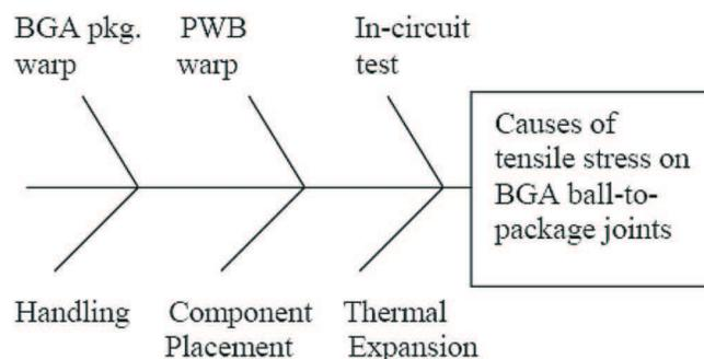
**Figure 13. Fishbone Diagram of Major Causes of Stress on BGA Packages and Solder Joints**
