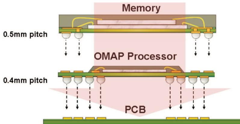
Figure 7. Assembly Options - 1 Pass
