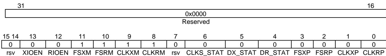
Table 1. Bit-Field Values for Pin Control Register
