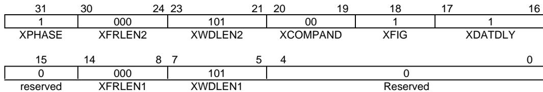
Table 2. Bit-Field Values for Receive/Transmit Control Register
